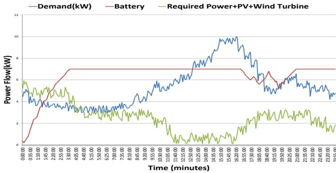
Fig. 9. Power flow after implementing predictive control algorithm.
