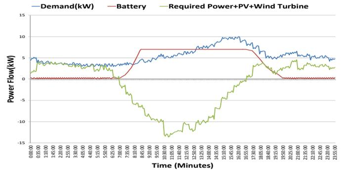
Fig. 8. Power flow before using predictive control algorithm.
