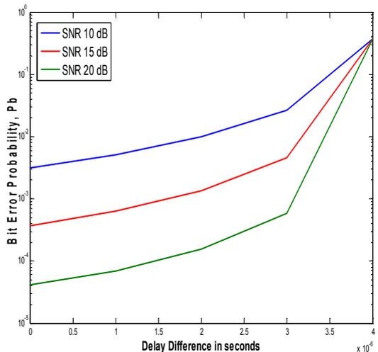
**Figure 3: BER versus transmission delay difference for a given SNR.**
