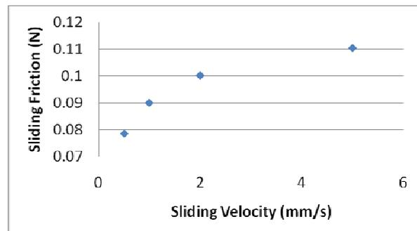
Fig. 2. The relationship between the sliding friction and the sliding velocity.
