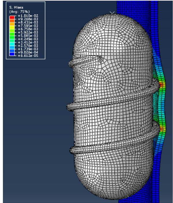
Fig. 5. The model in the 3D FE simulations.
