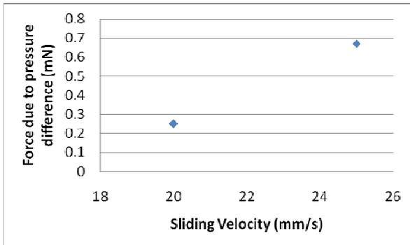
Fig. 4. The relationship between the force due to pressure difference and the sliding velocity, relatively high velocity..
