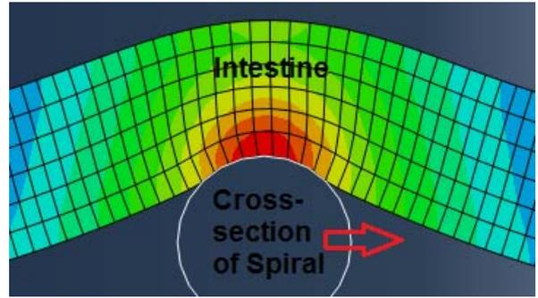
Fig. 1. The spiral sliding across the intestine in the 2D FE simulations.
