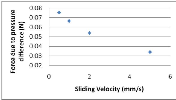
Fig. 3. The relationship between the force due to pressure difference and the sliding velocity, relatively low velocity.
