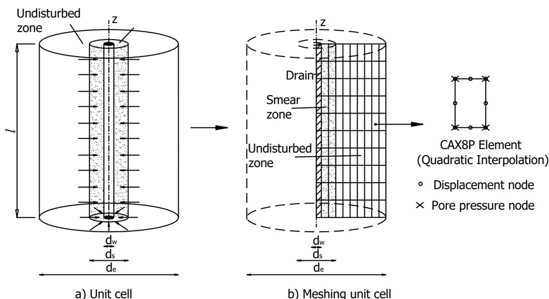
Fig. 2 Apply FEM to a model unit cell of vertical drain
