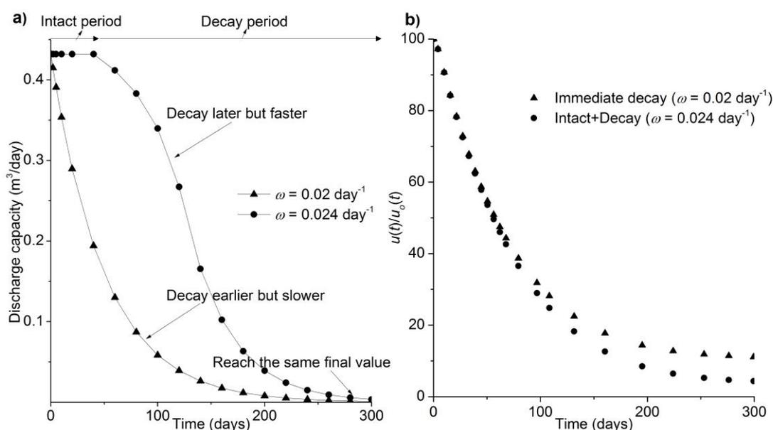
Fig. 5 Influence of difference in degradation of soil consolidation: a) immediate and late degradation of  $q_w$ ; and b) corresponding response of soil consolidation
