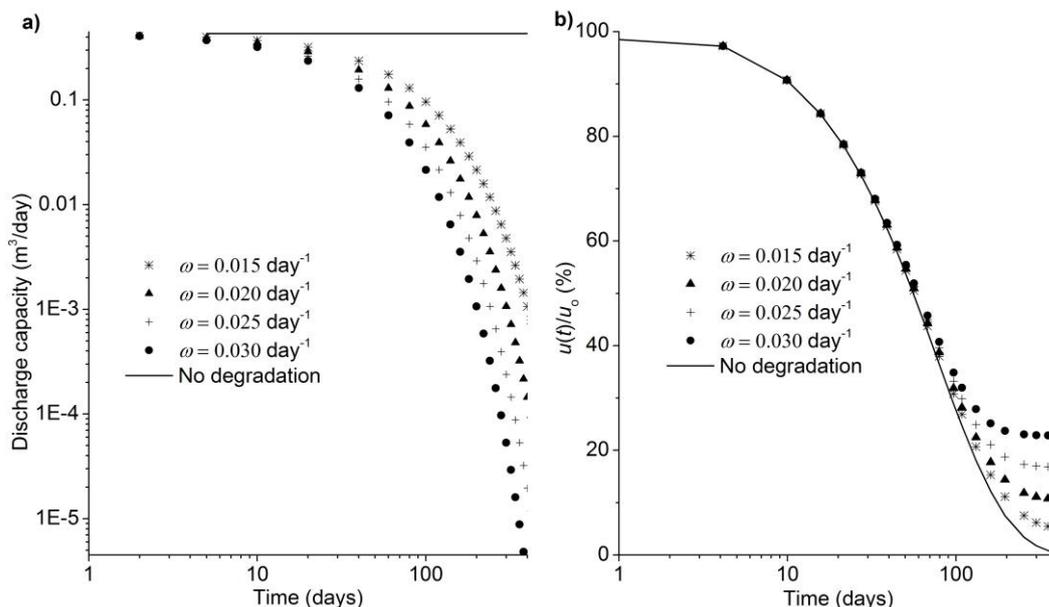
Fig. 4 Influence of drain degradation on soil consolidation: a) different rates of decay, and b) the corresponding consolidation of soil
