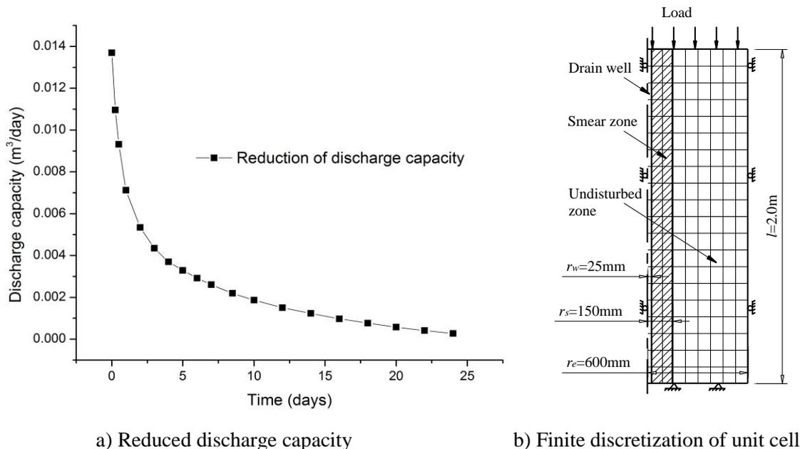
Fig. 6 FEM modelling degraded vertical drain conducted by Kim et al. [21]
