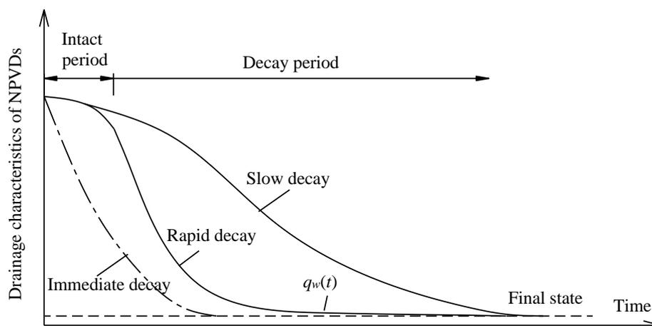
Fig. 1 Various types of degradation in the drainage characteristics of NPVDs
