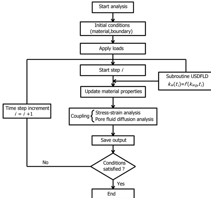
Fig. 3 Numerical scheme of FEM for analysing consolidation considering the degradation of drain
