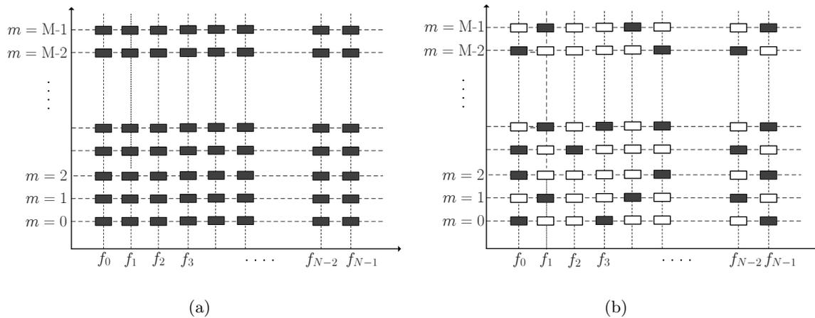
Figure 1. Data acquisition for TWRI: (a) conventional radar imaging scheme; (b) TWRI based on CS. The vertical axis represents the antenna location, and the horizontal axis represents the transmitted frequency. The filled rectangles represent the acquired data samples.
