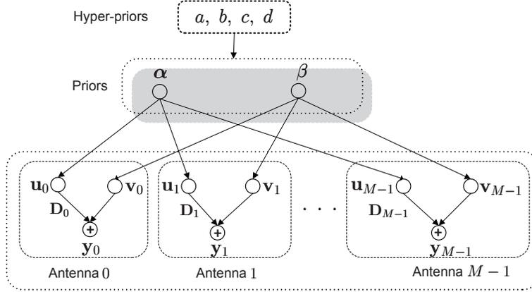
Figure 3. Hierarchical Bayesian model for the joint range profile reconstruction in the TWRI problem.
