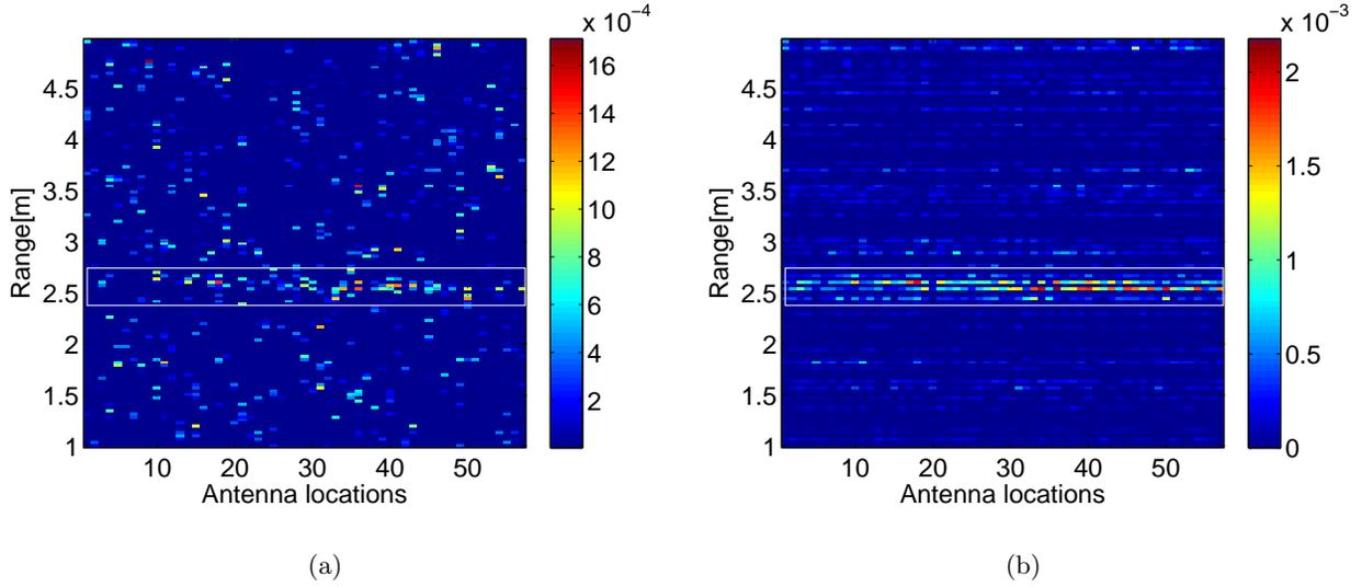
Figure 6. Comparison of the radar range profiles: (a) reconstructed by the conventional CS approach using 3% of full data samples; (b) reconstructed by the proposed JBCS approach using 3% of full data samples.
