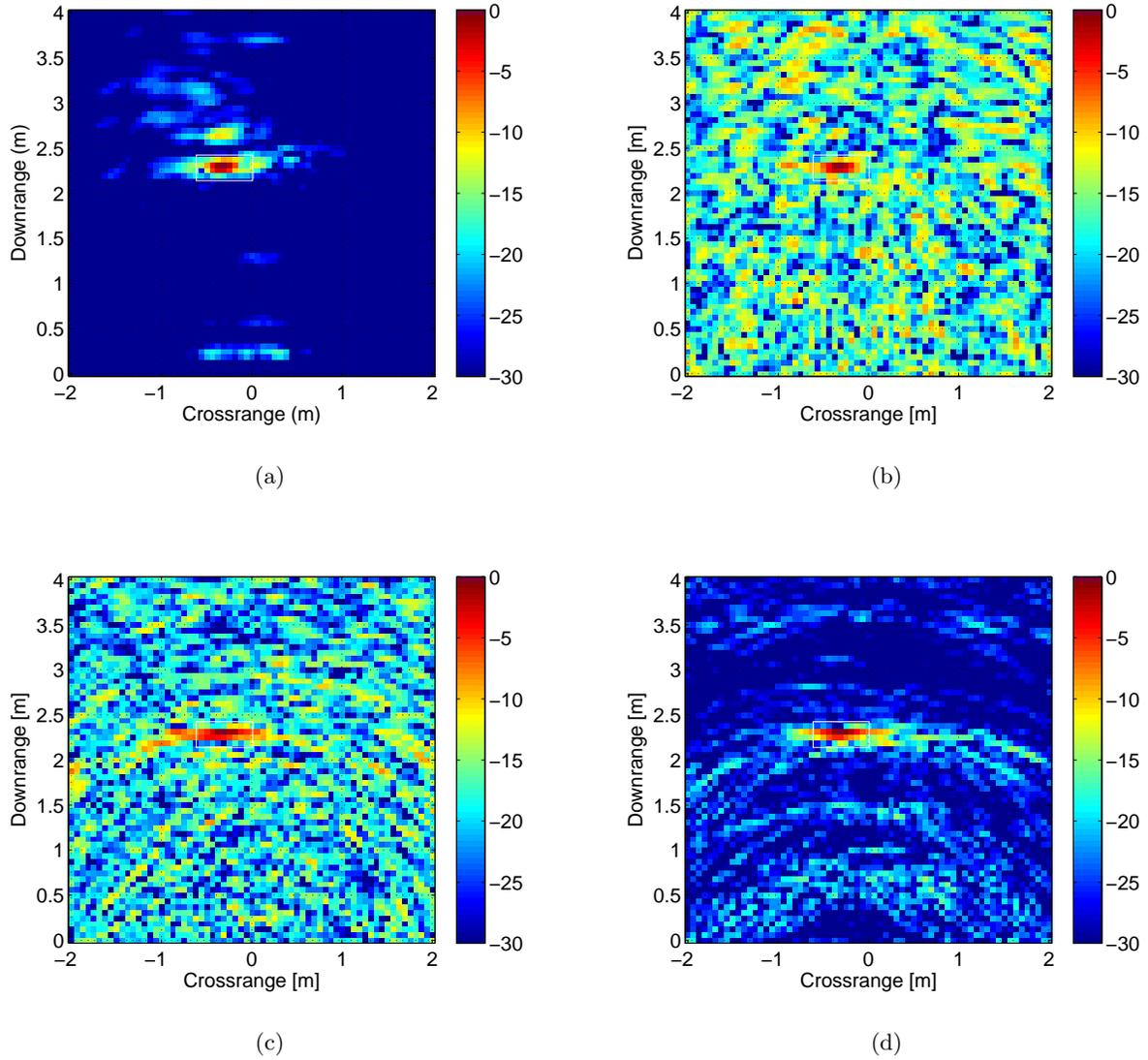
Figure 5. Images produced by different TWRI approaches (a) DS beamforming using full data samples (TCR = 54.23 dB); (b) DS beamforming using 3% of full data samples (TCR = 27.70 dB); (c) CS using 3% of full data samples (TCR = 30.08 dB); (d) proposed JBCS using 3% of full data samples (TCR = 43.38 dB).
