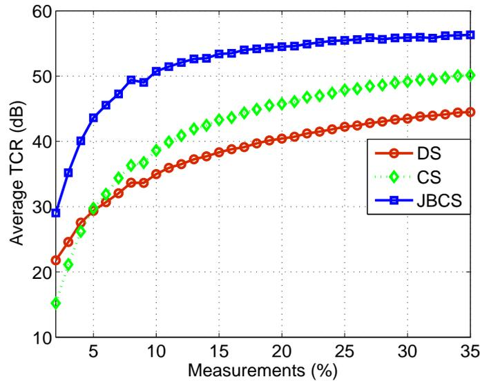
Figure 9. Comparison of the performance between the conventional DS beamforming, CS and the proposed JBCS approaches in terms of the average TCR of the formed images.
