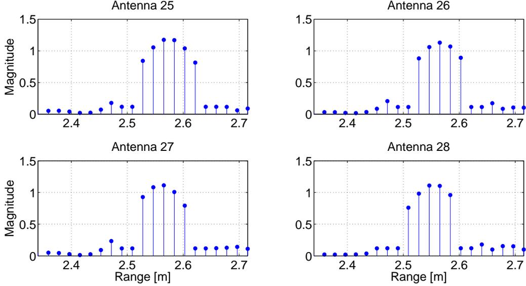
Figure 2. Range profiles computed using full data samples received at several antenna locations in the middle of antenna array.
