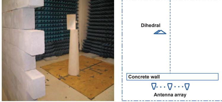
Figure 4. TWRI data acquisition. Left: a photo of the scene; Right: a top-view of the behind-the-wall scene.
