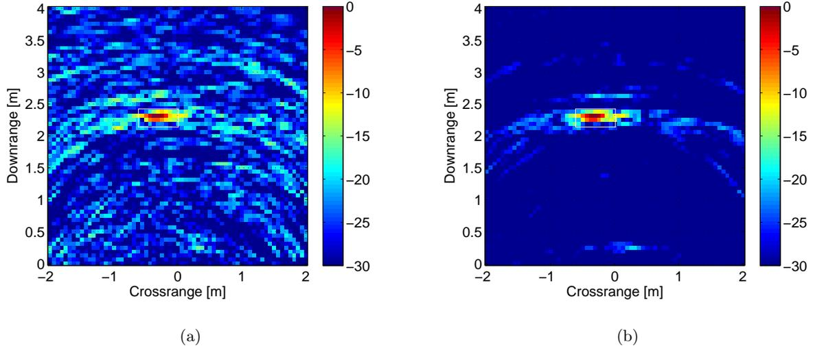
Figure 7. Images produced by different TWRI approaches: (a) the conventional CS approach (TCR = 42.58 dB); (b) the proposed JBCS approach (TCR = 54.72 dB). Here, 10% of the full data volume were used.
