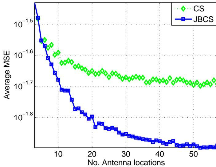
Figure 8. The average MSE of range profiles reconstructed by the conventional CS and the proposed JBCS approaches.
