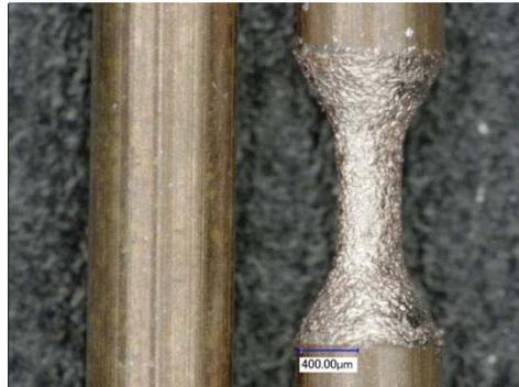
FIGURE 2. Deformed Specimen by MCWR.
