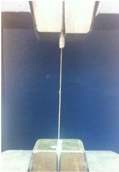
Figure 2. Tension test on single fibre
