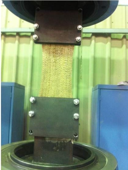
Figure 9. Tension test on the whole drain
