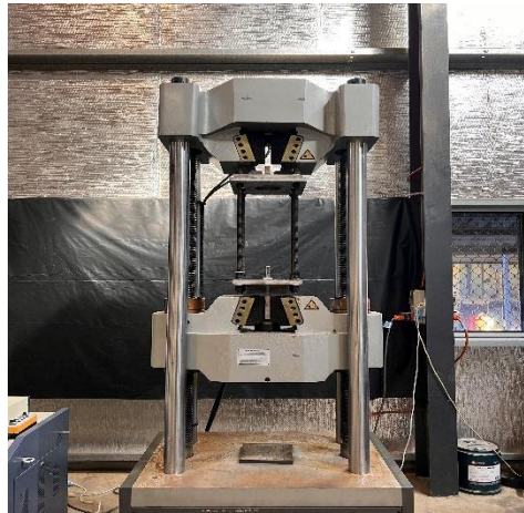
Figure 3: 100kN compression testing machine
