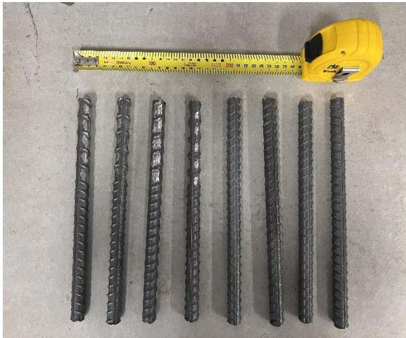
Figure 1: Rebars with two different rib space
