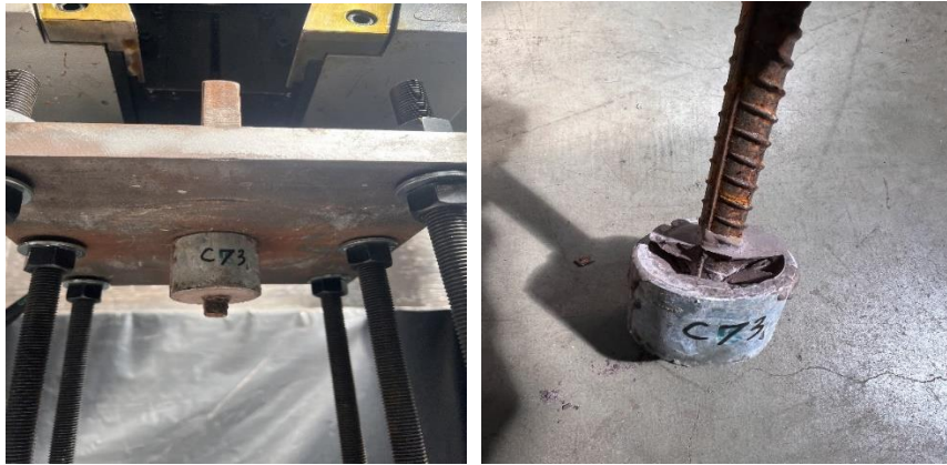
Figure 5: 7days old sample after pull-out test
