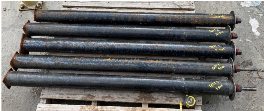
Figure 5: Bolt tail length for 10 second (Bolts 1 to 3) and 5 second (Bolts 4 and 5) rotation cure time before applying pre-tension to the bolt nut
