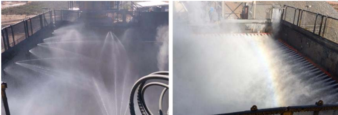
Figure 1: Example of a typical ROM bin with coarse (left) and fine (right) droplet spraying systems (Roberts and Wypych, 2017)
