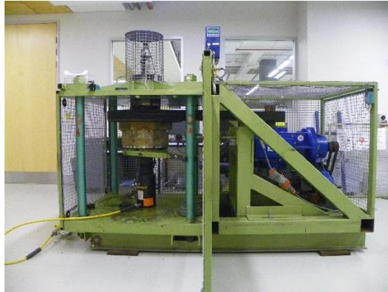
**Figure 1.** Photo of slow bearing lab test rig [6].
