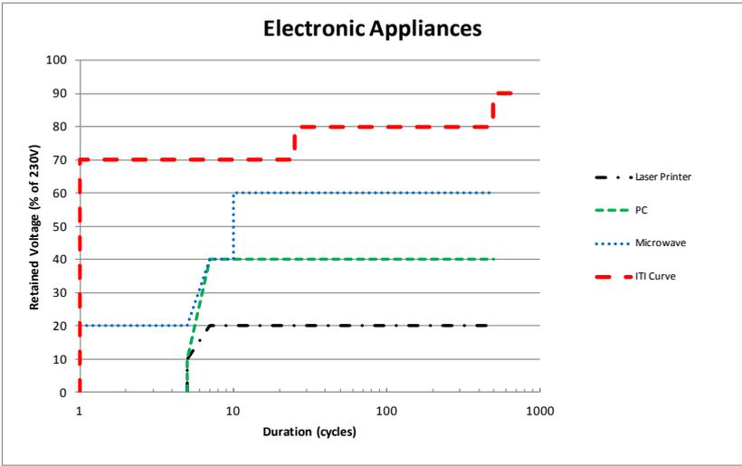
Figure 2. Sag Susceptibility Curves for Selected Electronic Equipment
