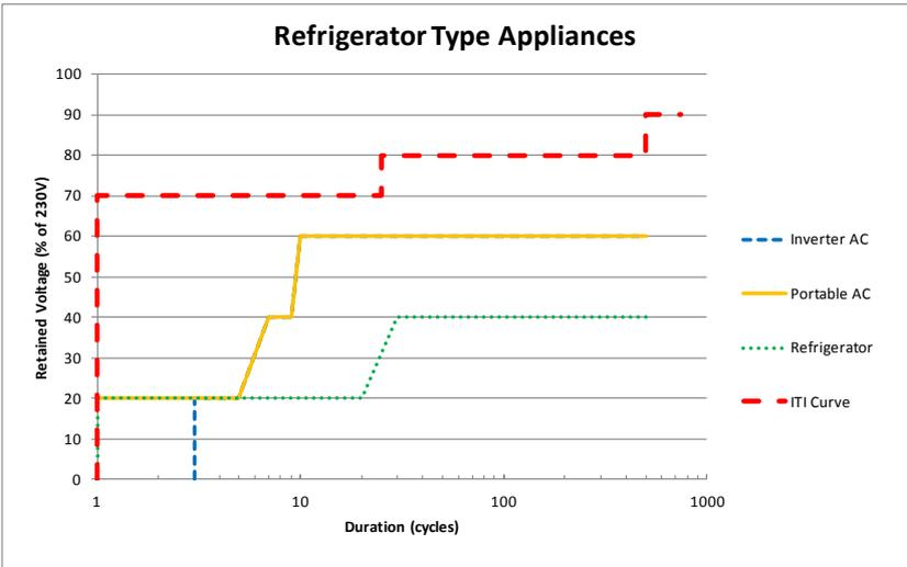
Figure 4. Sag Susceptibility Curves for Refrigerator Type Equipment
