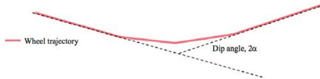
Fig. 2. Wheel-rail trajectory over a dipped rail joint.
