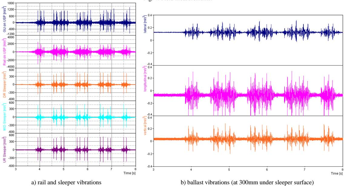
Fig. 5. Vibration attenuation through under sleeper pads.
