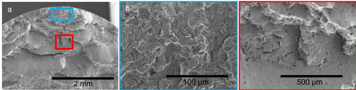
**Figure 2: Fracture surface of failed coupon; a) fracture surface overview; b) high magnification image on fracture origin (blue box in a); c) high magnification image on fast**
