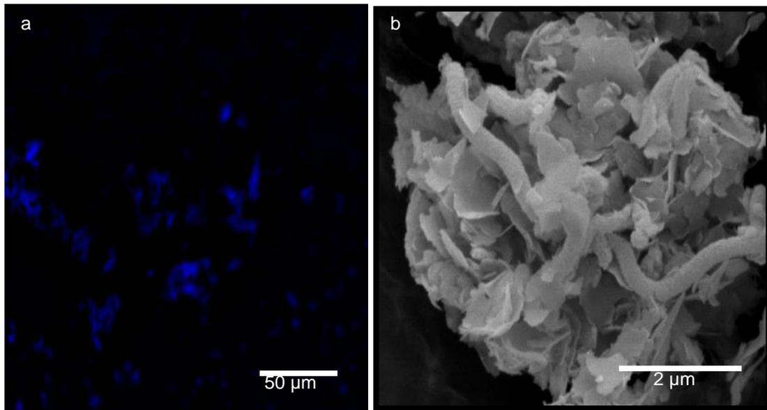
Figure 4: a) Biomass on the coupon surface; b) SEM image of detached biomass.
