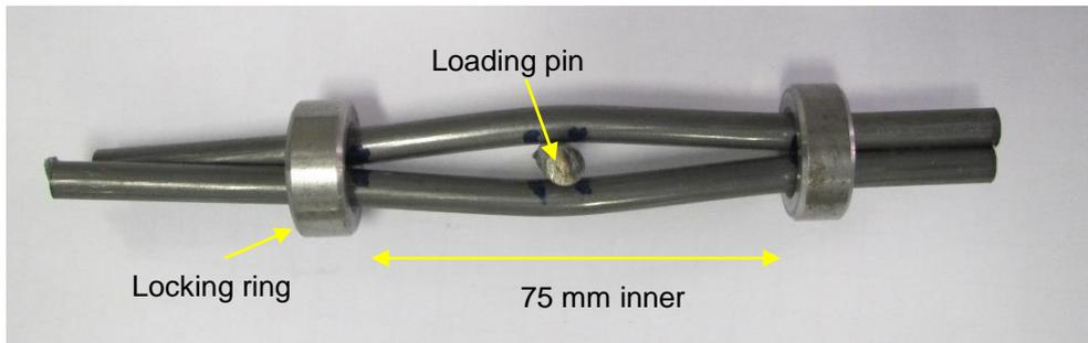
**Figure 1: Design of coupon.**
