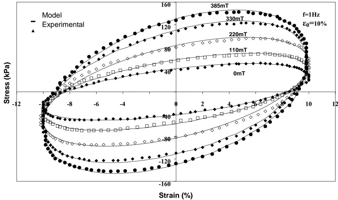
Fig. 7. A comparison between experimental data with model-predicted results with the amplitude input of 10%.
