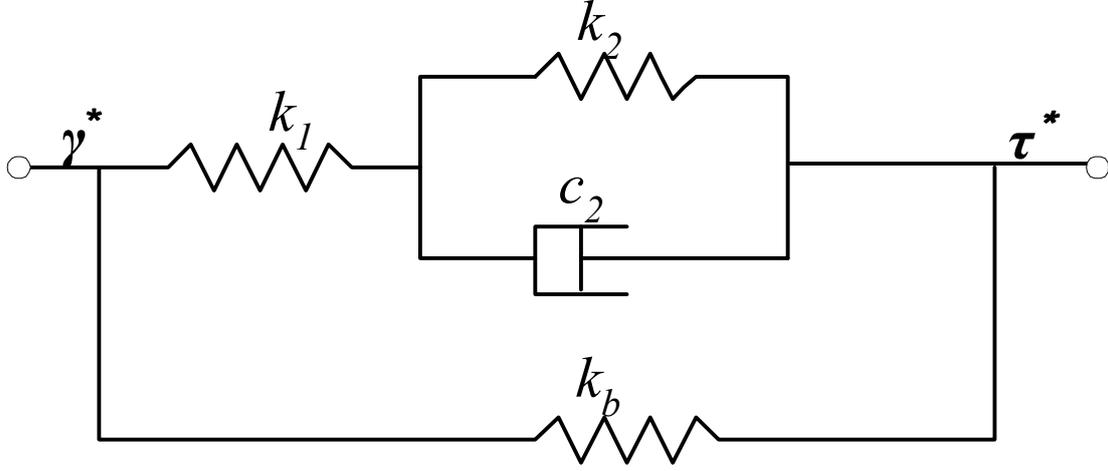
Fig. 6. Four-parameter viscoelastic model for MR elastomers.
