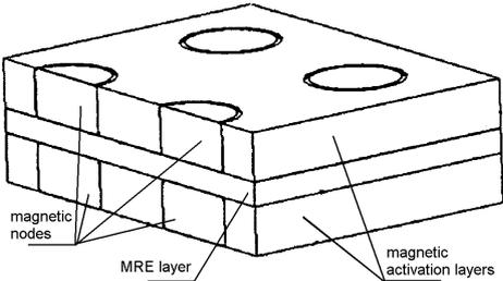
Figure 11. MRE devices for shock isolation [42,43]
