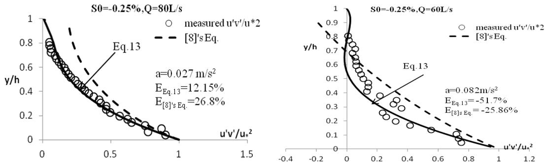
Figure 5: Comparison of measured and predicted Reynolds shear stress profile in accelerating steady flow based on [8] experimental data.
