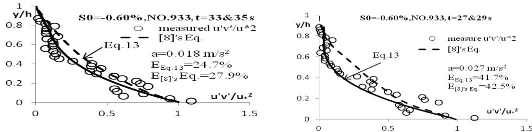
Figure 4: Comparison of measured and predicted Reynolds shear stress profile in accelerating unsteady flow based on [8] experimental data.
