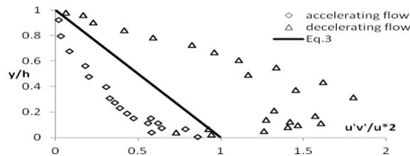
Figure 1: The measured Reynolds shear stress in uniform and non-uniform flows.
