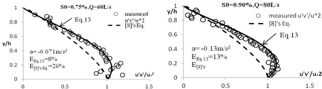
Figure 6: Comparison of measured and predicted Reynolds shear stress profile in decelerating steady flow based on Song’s (1994) experimental data.
