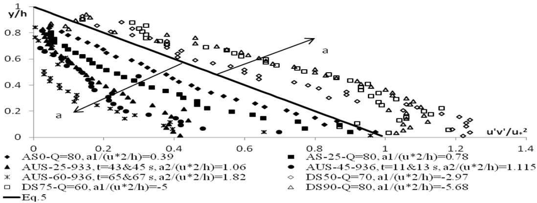
Figure 2: The influence of dimensionless flow acceleration on the deviation of measured Reynolds shear stress in accelerating and decelerating steady and unsteady flows from uniform flow based on [8] experimental data sets.
