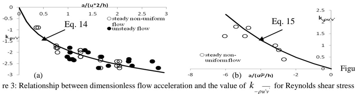
Figure 3: Relationship between dimensionless flow acceleration and the value of  $k_{-\rho u'v'}$  for Reynolds shear stress  $(-\overline{u'v'})/u_*^2$  in (a) accelerating and (b) decelerating steady and unsteady flow based on selected data sets from [8] experimental data.
