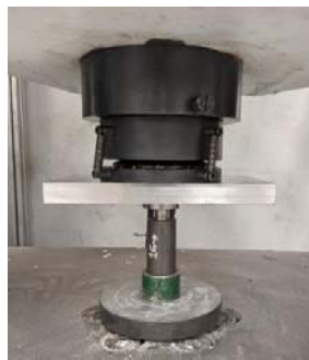
Figure 1: Push test setup
