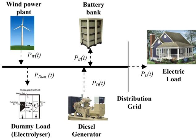
Figure 5. General model of a wind-battery-diesel plant
