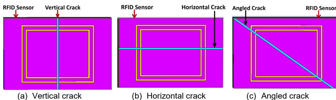
**Figure 9: RFID sensor with different crack orientation**
