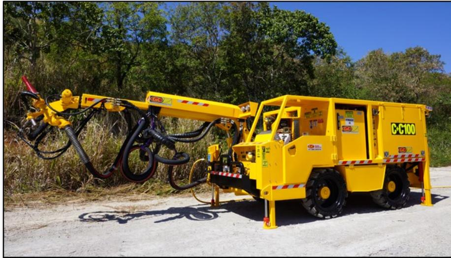
**Figure 1: Flameproof Shotcrete Rig (FSR)**
