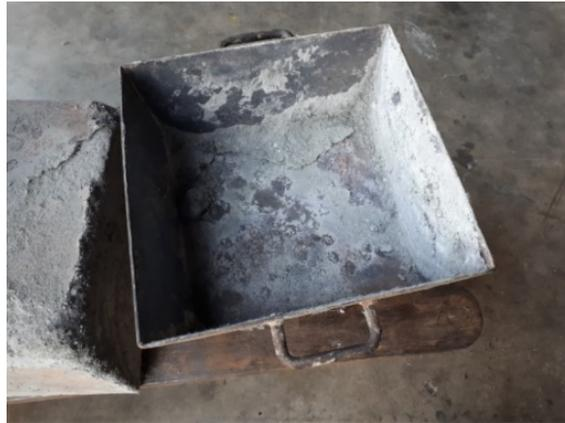
**Figure 43: 400mm x 400mm Core Panel Box**
