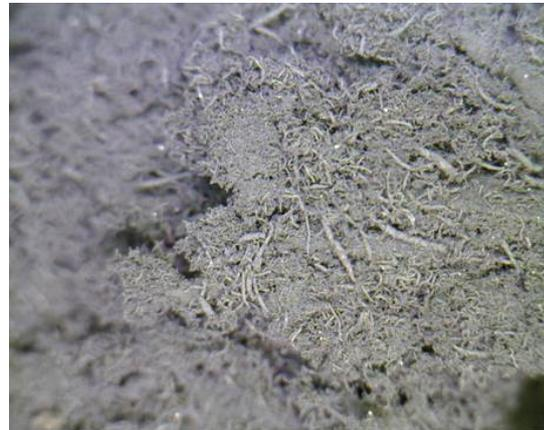
Figure 4: Digital microscope image of CBRF
