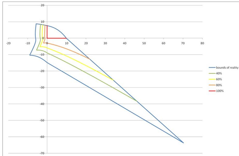
Figure 6: Explosibility safety margins for methane air mixes
