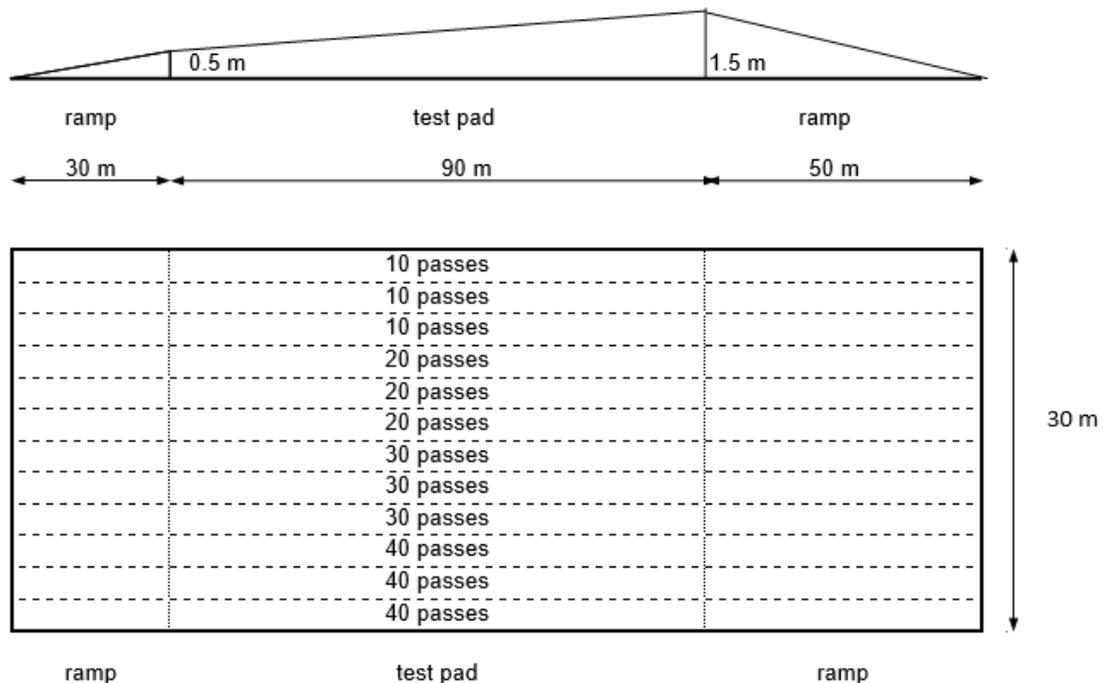
**Figure 2: Test pad for impact rolling trial**
