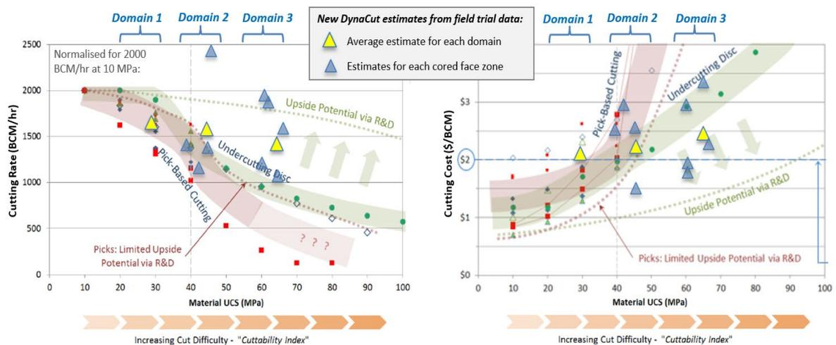
**Figure 5: Revised estimates of cutting rate (left) and cutting cost (right) for pick-based and undercutting disc technologies – based on new test results**
