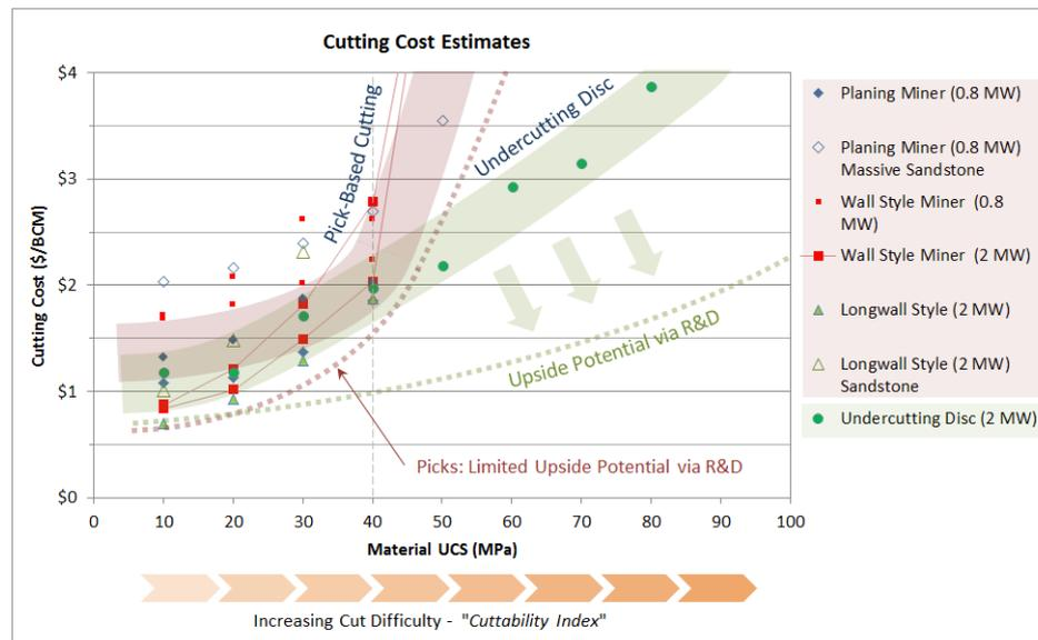
**Figure 2: Estimated cutting cost trends of current and emerging rock cutting technologies**
