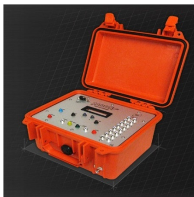
Figure 6: MicroTrap VOD recorder
