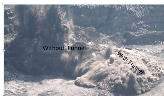
Figure 8: Fly rock generation
