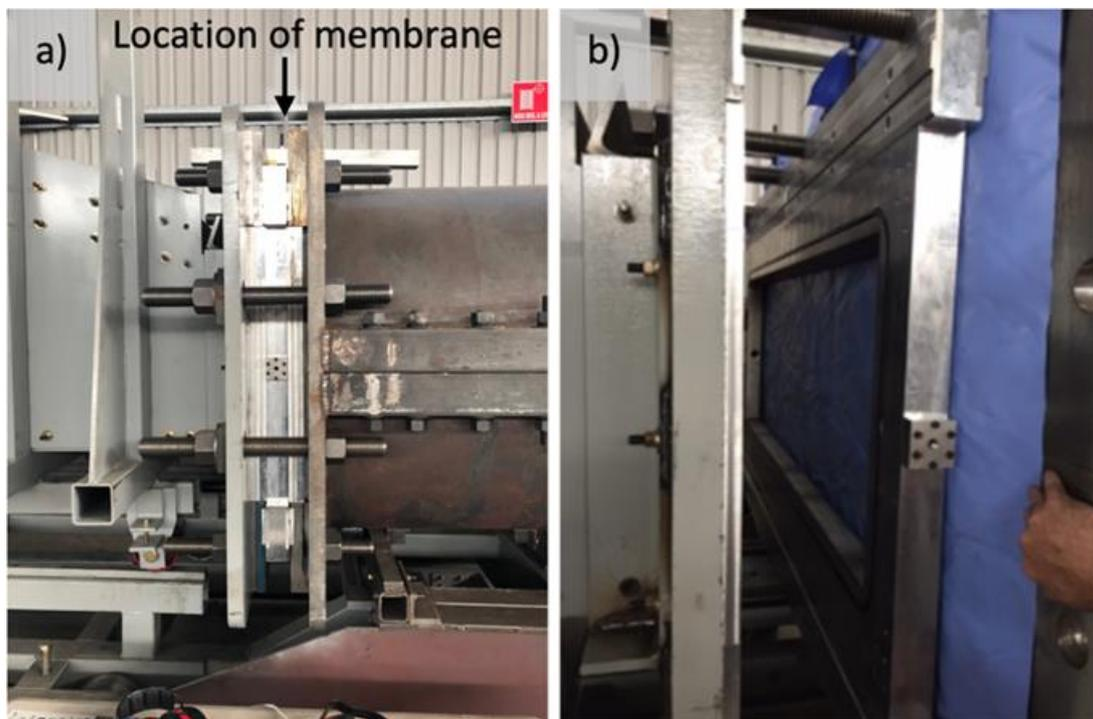
**Figure 3: Compressed gas Driver mode: a) Location of membrane (i.e. diaphragm station); b) Clamping of a frangible membrane across the opening of the Driver to create a gas tight barrier**
