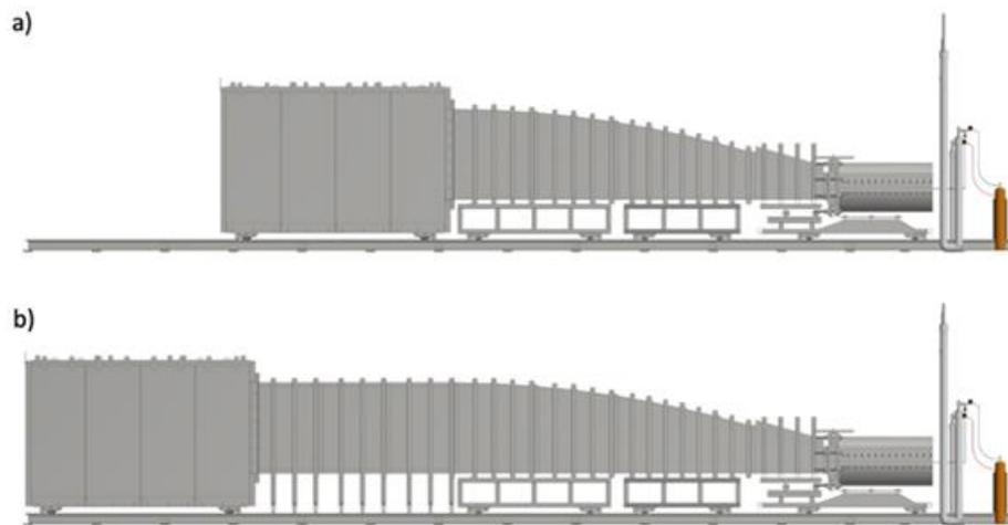
**Figure 5: Modular design allows for adjustment of standoff distances: a) Reduced standoff distance; b) Full standoff distance**
