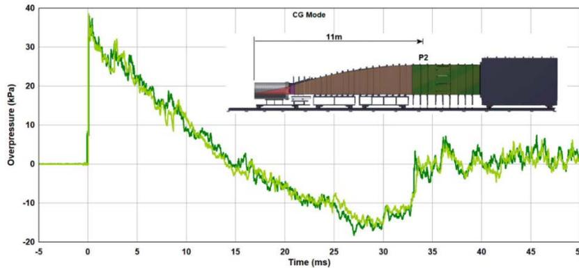
Figure 10: Waveform generated using 260 kPa compressed-air CG Driver showing two test results overlaid
