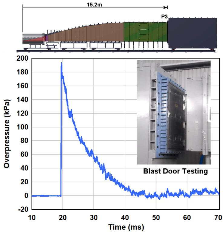
Figure 9: Reflected blast loading on a target door mounted to the front of the Reaction Housing for 0.14 m<sup>3</sup> oxy-acetylene GD Driver
