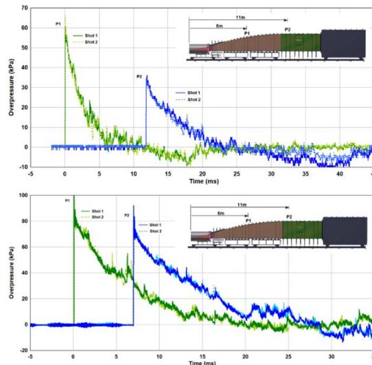
**Figure 8: [Upper] Waveform generated using 0.071 m<sup>3</sup> oxy-acetylene GD Driver showing results for two tests overlaid; [Lower] waveform generated using 0.14 m<sup>3</sup> oxy-acetylene GD Driver showing two test results overlaid**
