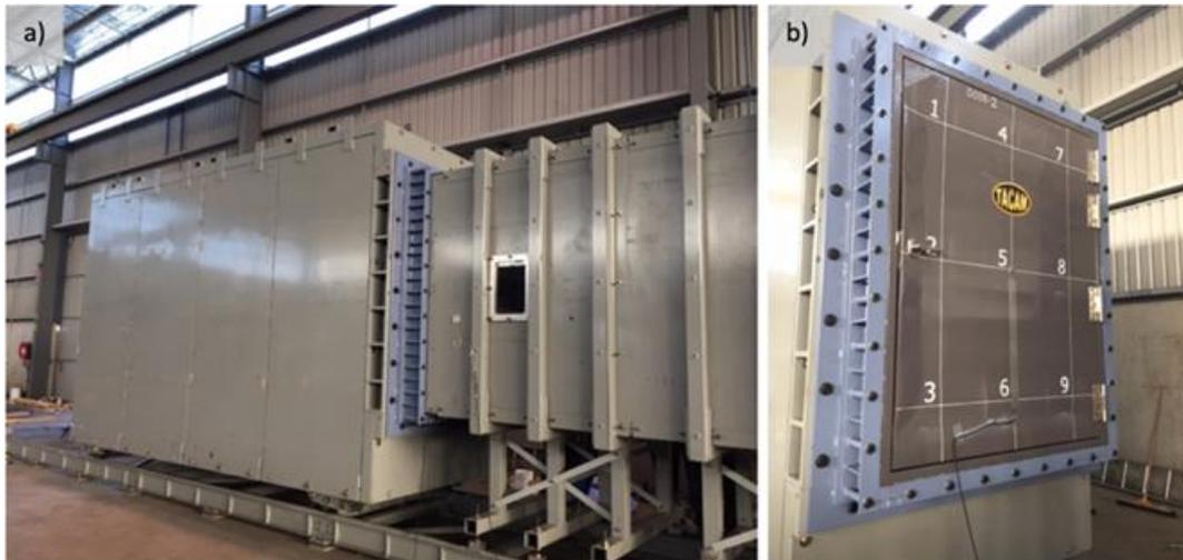
**Figure 7: Mounting of reflective targets: a) Reaction Housing with a reflective target in pre-testing position; b) Test specimen mounted on Reaction Frame**
