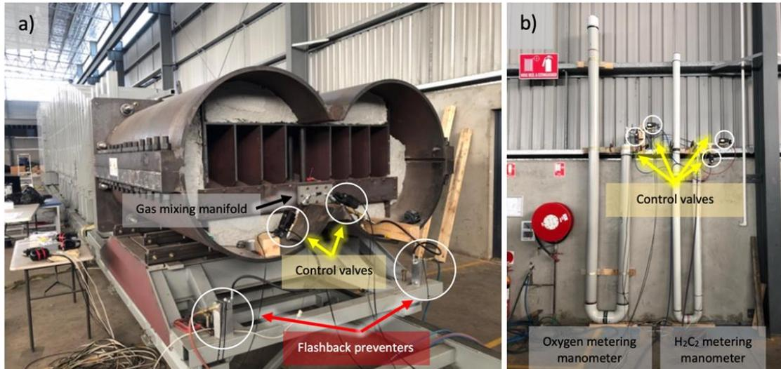
**Figure 4: Gaseous detonation Driver mode: a) Flammable gas delivery system; b) Manometers for precise metering of combustion gases**
