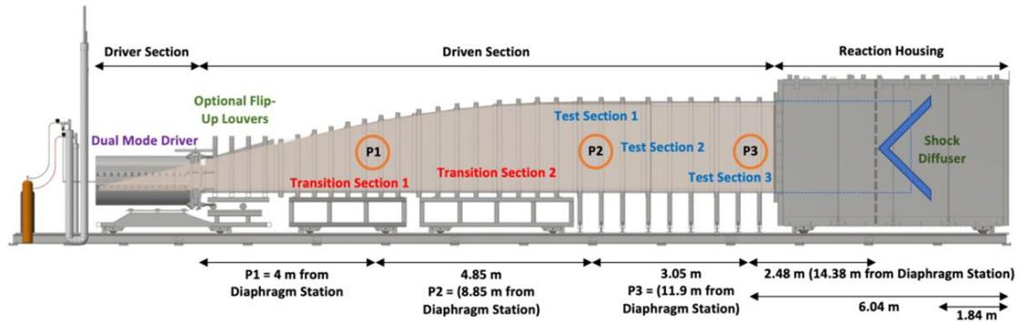
**Figure 2: Schematic of NFPBS Advanced Blast Simulator (ABS)**
