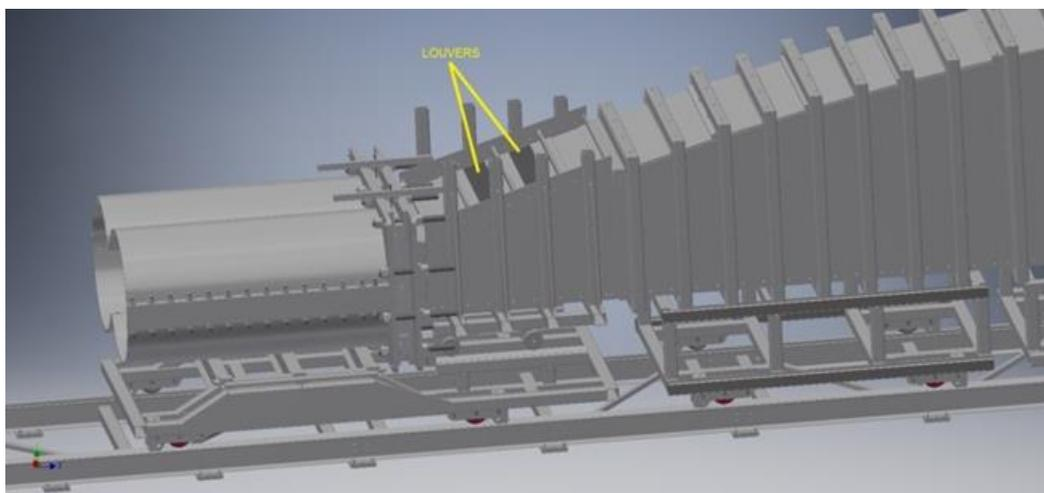
**Figure 6: Flip-up louvers to allow for controlled venting of reflecting shock waves reflecting back from reflective targets**
