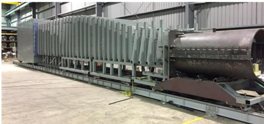
**Figure 1: NFPBS Advanced Blast Simulator (ABS) configuration as-built**
