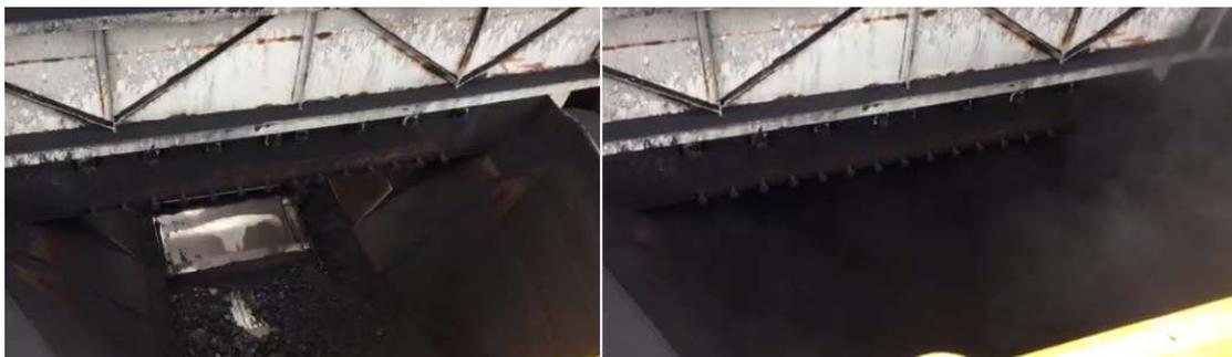
**Figure 4: Dust escaping through opening for feeder**
