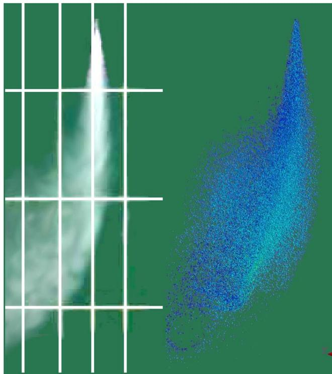
**Figure 2: Actual Spray (Left) and Simulated Spray (Right)**
