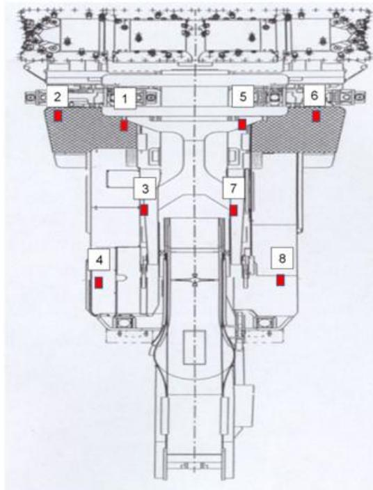
**Figure 3: Pump and head placement on MB650**
