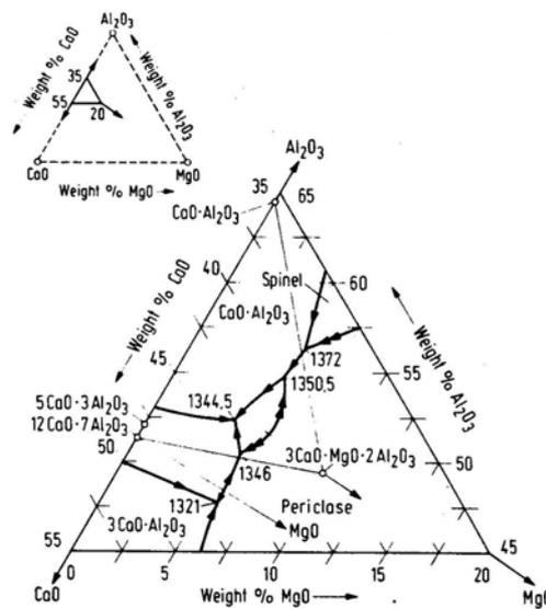
Fig.3: Ternary phase diagram of CaO-Al<sub>2</sub>O<sub>3</sub>-MgO[6]
