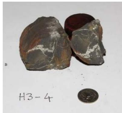
**Figure 4: Photograph of siderite nodules containing marcasite/pyrite stringers**
