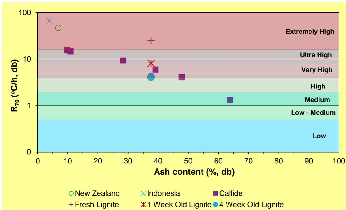
**Figure 1: Relationship between R<sub>70</sub> self-heating and ash content showing intrinsic spontaneous combustion propensity ratings**
