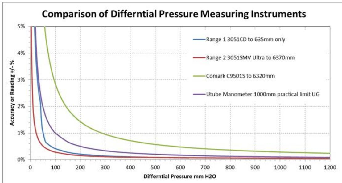
Figure 1: Comparison of differential pressure measuring instruments
