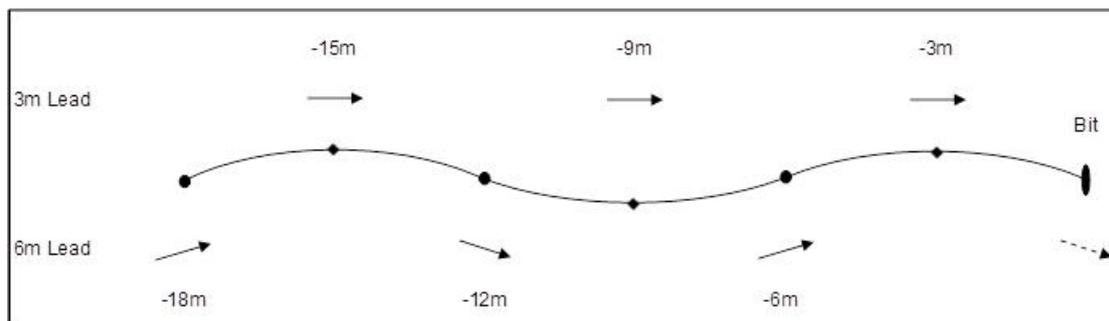
**Figure 1: Survey positions with 6 m orientation changes**
