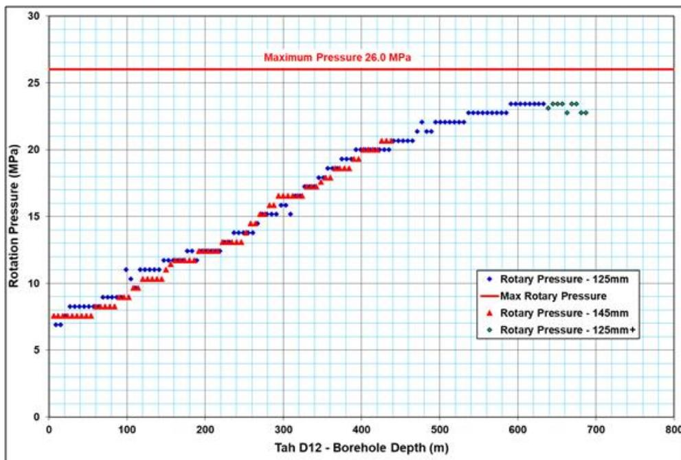
Figure 11: Rotational pressure of over-core drilling
