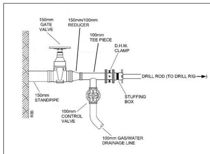
**Figure 2: Standpipe configuration with 150 mm to 100 mm reduction**
