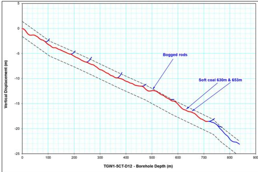
**Figure 8: Profile of bogged rods**
