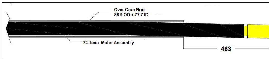
**Figure 4: Wash over comparison of HQ drill rods with 93 mm diameter DHM (REI/DPI, 2012)**
