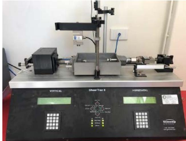
**Figure 3: Fully automated direct shear testing machine**
