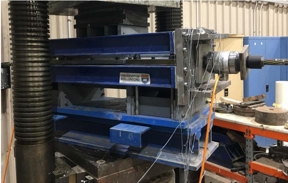
Figure 5: test sample installation and strain gauges connecting monitor channels
