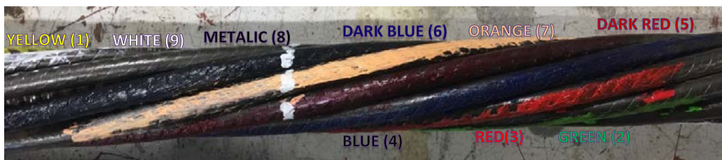
4a: Colour painted on cable bolt
