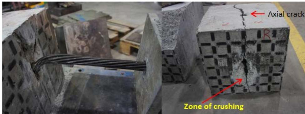
**Figure 3: Cracked concrete block after shearing and zone of crushing****MK-IV CIRCULAR DOUBLE SHEAR BOX (NAJ AZIZ DOUBLE SHEAR BOX)**
