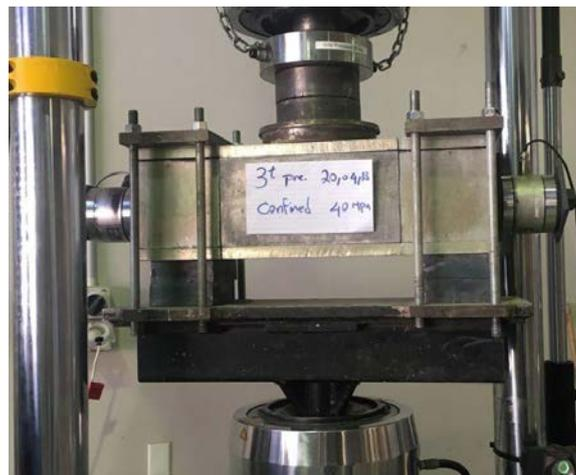
Figure 1: MKI double shear rig
