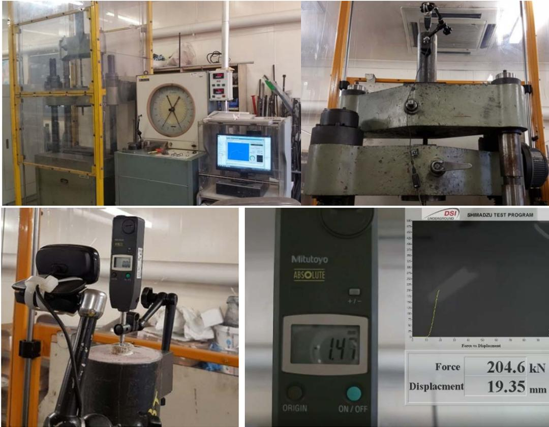
**Figure 6: Pull-test arrangement on Universal Test Machine (UTM)**
