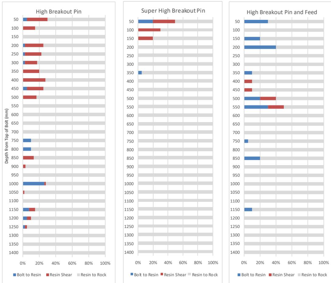
**Figure 9: Resin failure mode by 50mm increment along the bolt**
