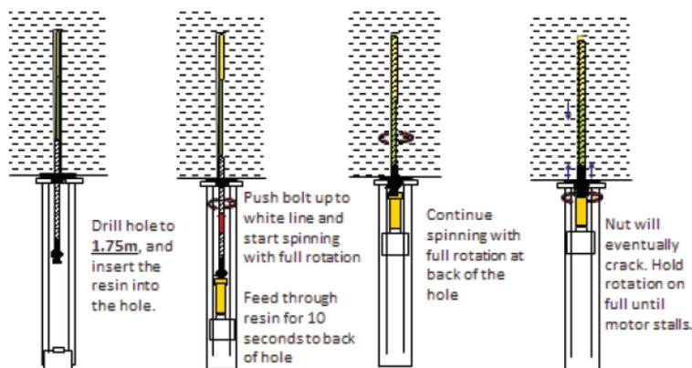
**Figure 2: Spin-to-stall installation procedure (from Emery, et al 2015)**
