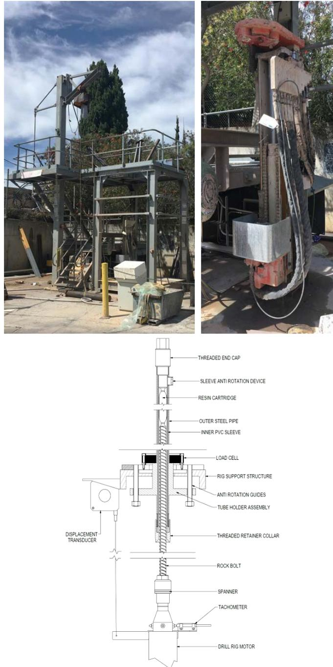
**Figure 4: Drill rig facility at DSI Underground**
