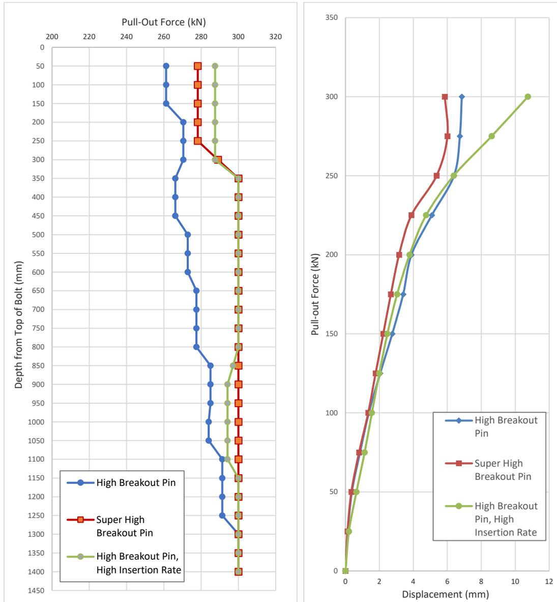
**Figure 8: (a) pull-out force by depth along the bolt (left), and (b) pull-out load and displacement for the three test specifications**
