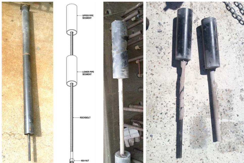
**Figure 5: Spin-to-stall test samples**
