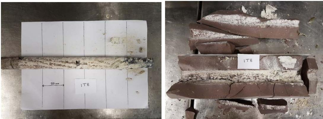
**Figure 7: Example observation of resin-anchor defects and mode of resin bond failure**
