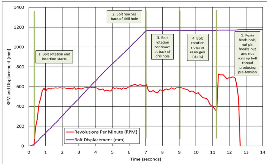
**Figure 3: Drill rig instrumentation showing a typical spin-to-stall resin bolt installation**
