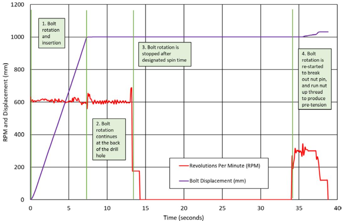
**Figure 1: Drill rig instrumentation showing a typical spin-and-hold resin bolt installation**
