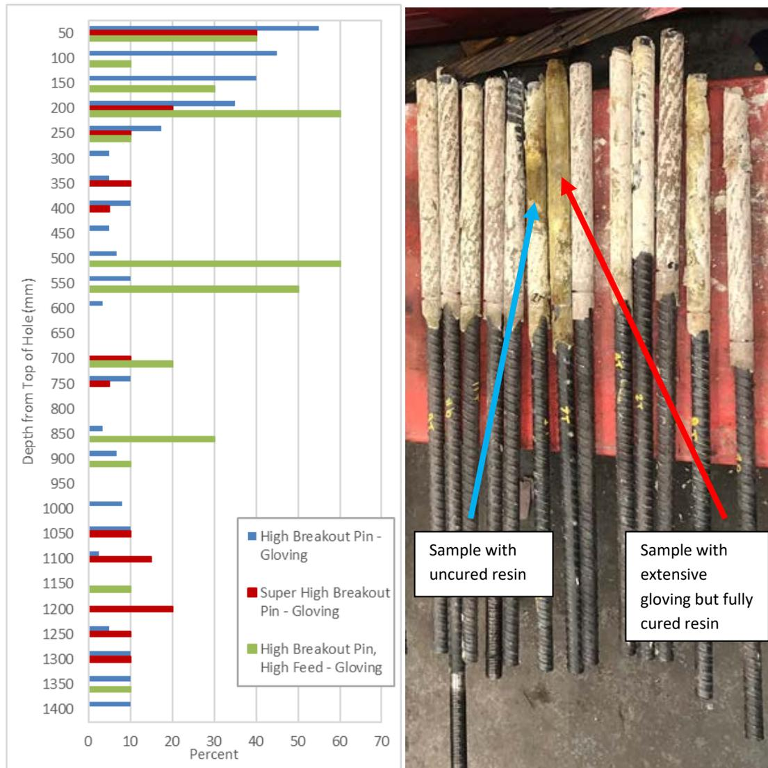
**Figure 10: (a) Proportion of gloving distributed along the bolt length, and (b) sample inspection after pull-out load testing**
