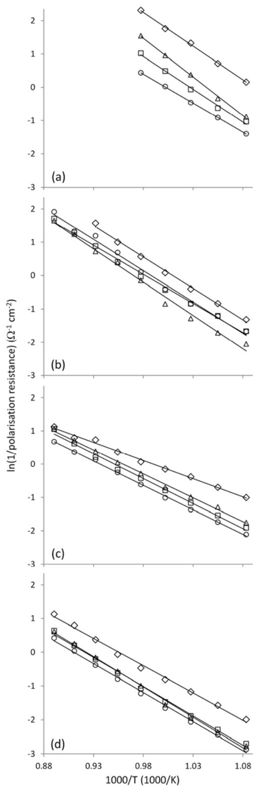
Fig. 7. Electrochemical oxygen reduction activity of  $(\text{La}_{0.8}\text{Sr}_{0.2})_{0.98}\text{Cr}_x\text{Mn}_{1-x}\text{O}_3$  model series in air over the temperature range 850-650 °C. (a) process A,B, (b) process  $\text{C}_1$ , (c) process  $\text{C}_2$ , (d) overall oxygen reduction reaction. ( $\diamond$ )  $x = 0$ , ( $\square$ )  $x = 0.02$ , ( $\circ$ )  $x = 0.05$ , ( $\Delta$ )  $x = 0.1$ .
