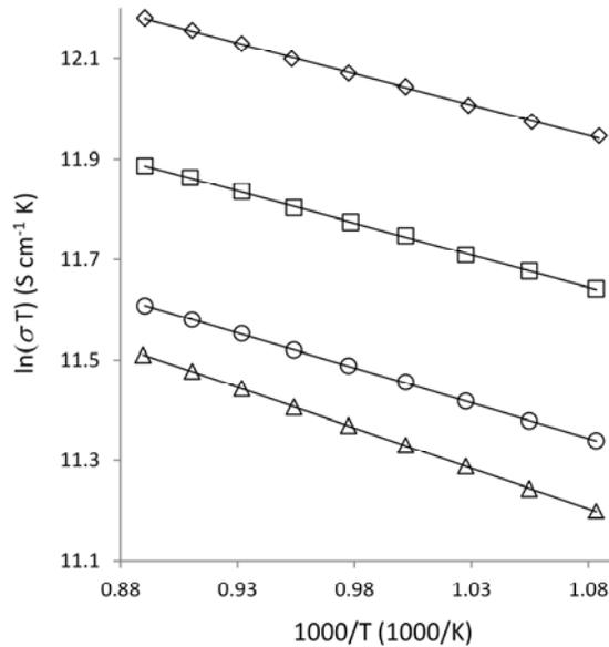
Fig. 2. Electronic conductivity ( $\sigma$ ) of  $(\text{La}_{0.8}\text{Sr}_{0.2})_{0.98}\text{Cr}_x\text{Mn}_{1-x}\text{O}_3$  pellets measured in air between 850-650 °C using the van der Pauw method. ( $\diamond$ )  $x = 0$ , ( $\square$ )  $x = 0.02$ , ( $\circ$ )  $x = 0.05$ , ( $\Delta$ )  $x = 0.1$ .
