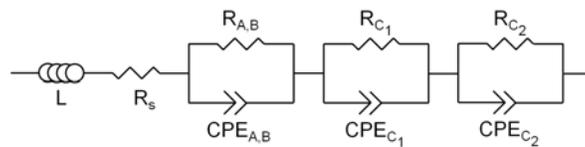
Fig. 4. Equivalent circuit used to fit electrochemical impedance spectroscopy data obtained for symmetrical cells based on the  $(La_{0.8}Sr_{0.2})_{0.98}Cr_xMn_{1-x}O_3$  model series.
