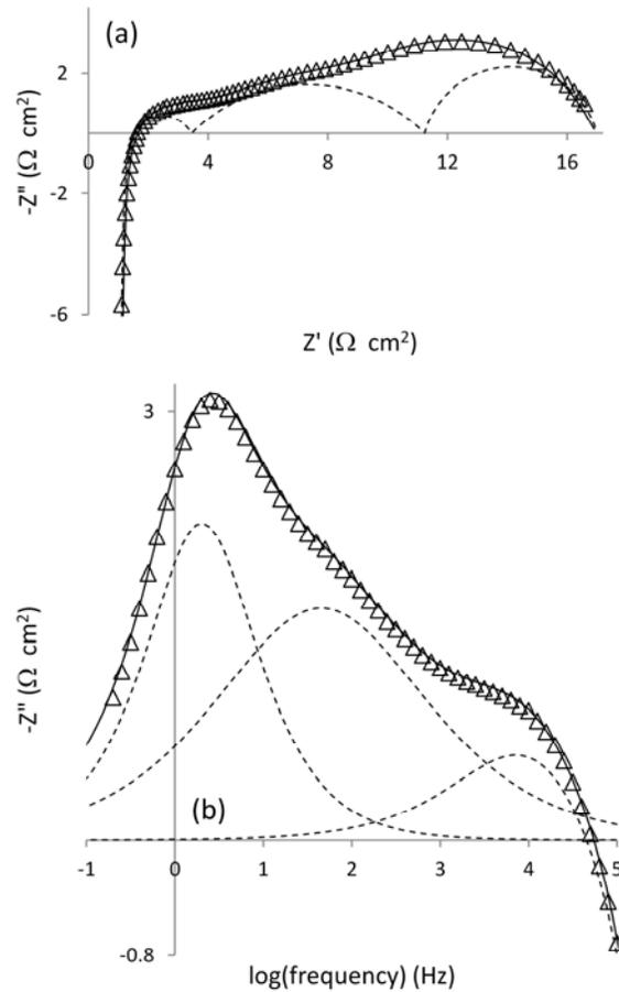
Fig. 5. Example deconvolution and overall fitting of (a) Nyquist and (b) Bode plots measured in air at 650 °C for a symmetrical cell based on  $(\text{La}_{0.8}\text{Sr}_{0.2})_{0.98}\text{Cr}_{0.1}\text{Mn}_{0.9}\text{O}_3$ . ( $\Delta$ ) experimental data, (---) individual components of fit, (—) overall fit. Contribution of YSZ electrolyte, wires and contacts to ohmic resistance subtracted from data in (a).
