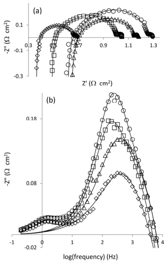
Fig. 6. Electrochemical impedance spectroscopy analysis in air at 850 °C of symmetrical cells based on  $(\text{La}_{0.8}\text{Sr}_{0.2})_{0.98}\text{Cr}_x\text{Mn}_{1-x}\text{O}_3$  model series. (a) Nyquist plot. (b) Bode plot. ( $\diamond$ )  $x = 0$ , ( $\square$ )  $x = 0.02$ , ( $\circ$ )  $x = 0.05$ , ( $\Delta$ )  $x = 0.1$ . Overall fits indicated by solid lines. Contribution of YSZ electrolyte, wires and contacts to ohmic resistance subtracted from data in (a).
