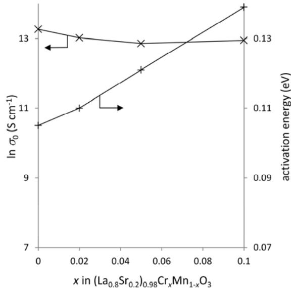
Fig. 3.  $\ln \sigma_0$  (x) and activation energy (+) from Fig. 2  $\ln(\sigma T)$  vs.  $1000/T$  plots for the  $(\text{La}_{0.8}\text{Sr}_{0.2})_{0.98}\text{Cr}_x\text{Mn}_{1-x}\text{O}_3$  model series plotted against extent of chromium substitution ( $x$ ). Error bars (not shown) smaller than symbols.
