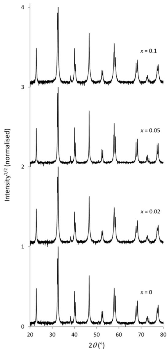
Fig. 1. X-ray diffraction patterns of  $(\text{La}_{0.8}\text{Sr}_{0.2})_{0.98}\text{Cr}_x\text{Mn}_{1-x}\text{O}_3$  powders prepared in air *via* solid state synthesis, with extent of chromium substitution ( $x$ ) as indicated.
