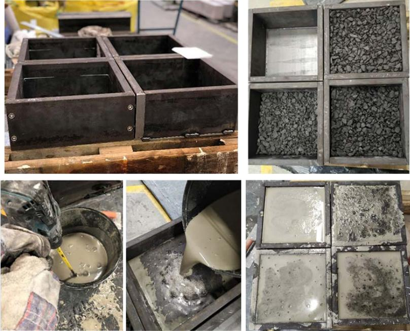
**Figure 2: Preparation of specimens**
