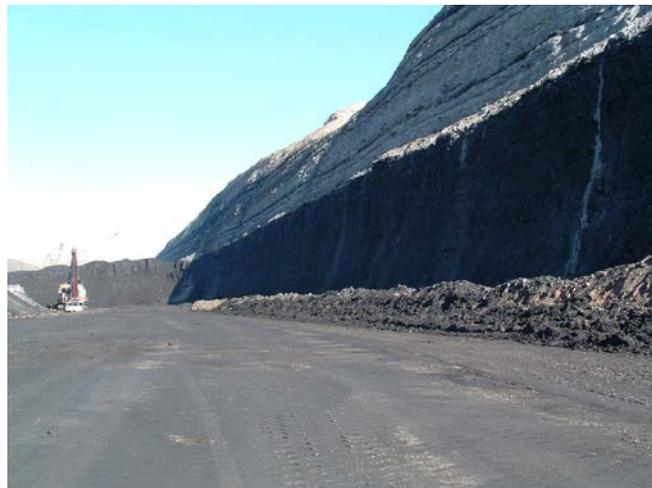
**Figure 3: Prepared Operating Bench with Berm and Drainage in Place**
