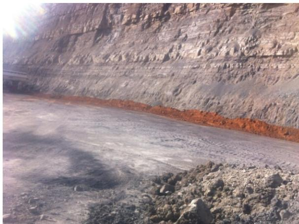
**Figure 9: Incident highwall – no berms and Ski Jump**
