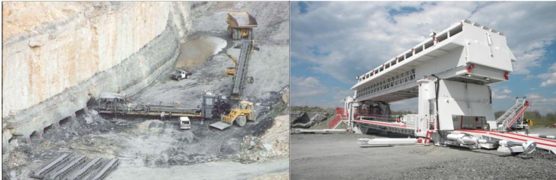
**Figure 1: The first Addcar system in 1990 and current Launch vehicle configuration**
