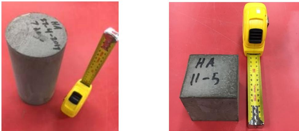
Figure 2: Prepared Samples [left] large scale cylinder UCS [right] small scale cube UCS
