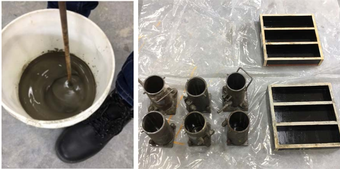
Figure 1: [left] Grout preparation [right] a view of large scale UCS and flexural moulds
