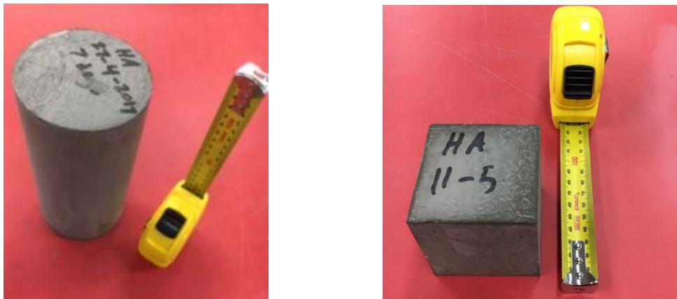
Figure 2: Prepared Samples [left] large scale cylinder UCS [right] small scale cube UCS
