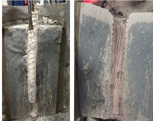
Figure 5: Typical failure in the weak confining medium at the grout/rock interface with the resin grout (left) and failure at the cable/grout interface with a cement grout (right).
