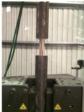
**Figure 11: Pull testing set up**
