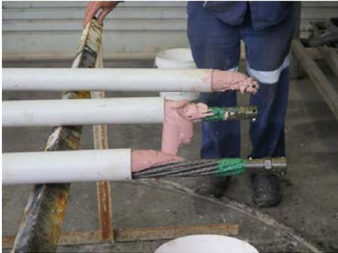
Figure 18: Full encapsulation of 6m cables
