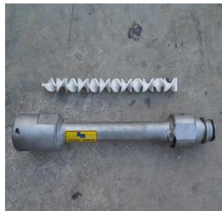
**Figure 17: Grout Static Mixer**
