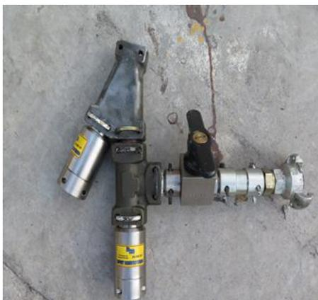
**Figure 16: Grout mixing attachment DN20 fittings**
