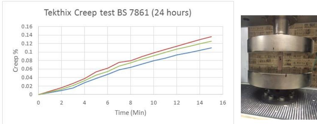
Figure 9: Rheological /Creep characteristic of Tekthix grout
