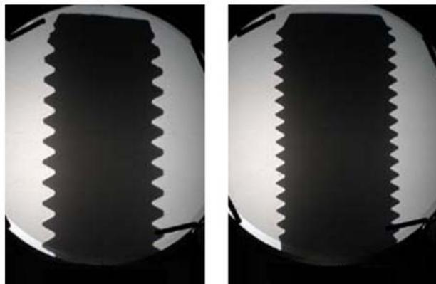
Figure 3: A coarse thread (left) and a fine thread (right)
