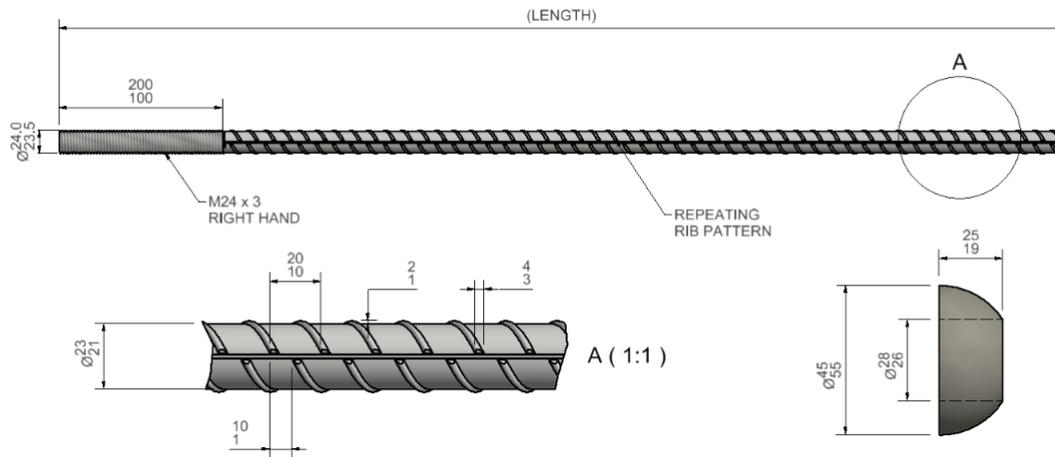
Figure 1: Typical Australian M24 rockbolt and dome ball washer dimensions
