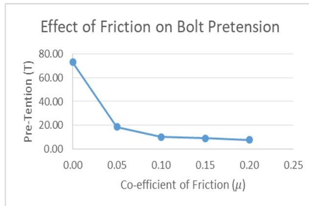
**Figure 4: Pre-tension achieved for various levels of friction for a 350 Nm input torque**
