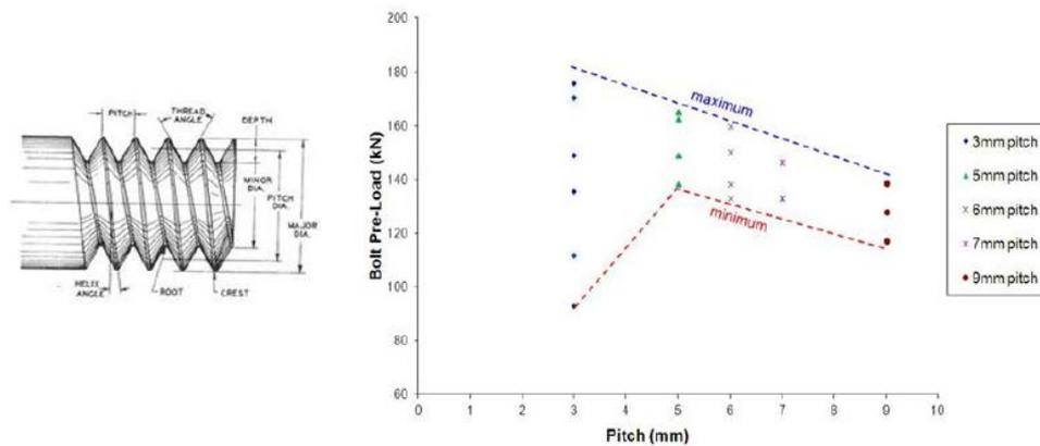
Figure 2: Impact of pitch height on pre tension values (Frith, 2017)
