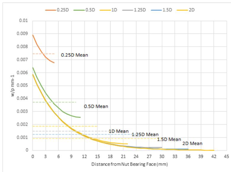
**Figure 5: Distribution of loading intensity along an M24 x 3 nut of varying lengths. Lengths are represented proportionally to the diameter of the thread (After Sopwith, 1948).**
