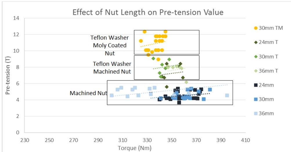
Figure 7: Torque v’s tension for 1D, 1.25D, 1.5D nut lengths with various friction reducing agents.
