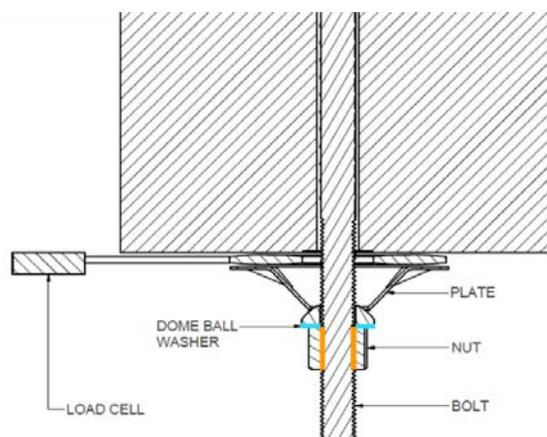
**Figure 6: Experimental setup highlighting major points of friction**
