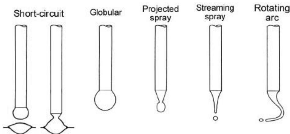
**Figure 1. Diagrammatic representation of transfer modes in argon-based shielding gases**
