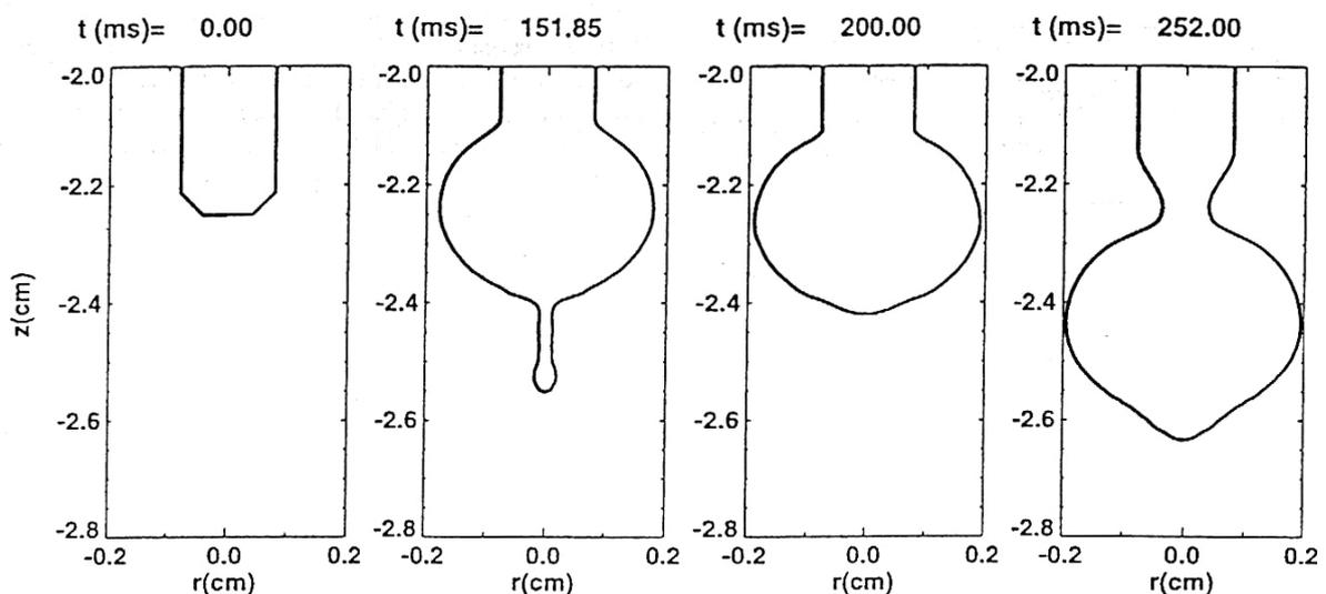
**Figure 2 Simulated droplet growth in pure CO<sub>2</sub> at 325A, 1.6mm electrode (from [12])**
