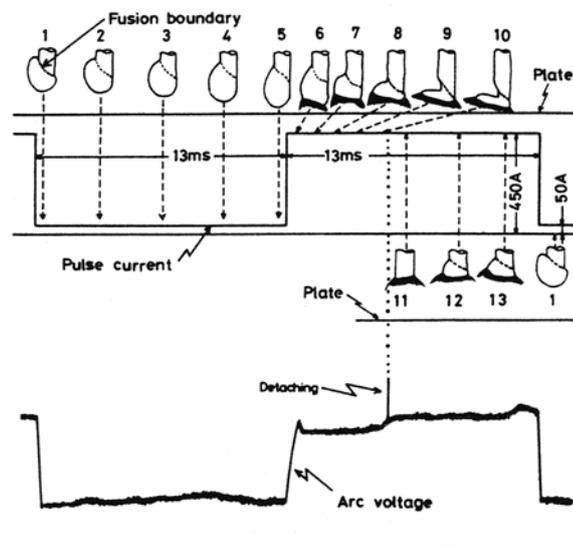
Figure 4 Example of droplet behaviour and waveforms in pulsed CO<sub>2</sub> (from [15])
