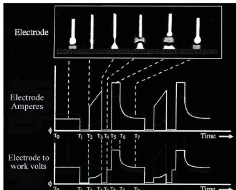
Figure 7 Current and voltage waveforms for power source of [4]
