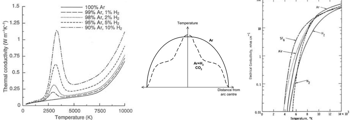
**Figure 3 (a) K vs T for Ar and Ar-H<sub>2</sub> mixtures (b) Changes in arc temperature distribution (c) Electrical conductivity vs T of various gases (courtesy J.J. Lowke)**
