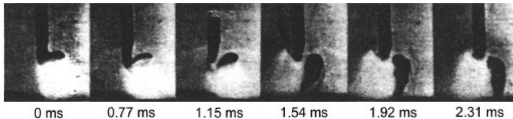
Figure 5 High speed cinematography of droplet transfer (from [15])
