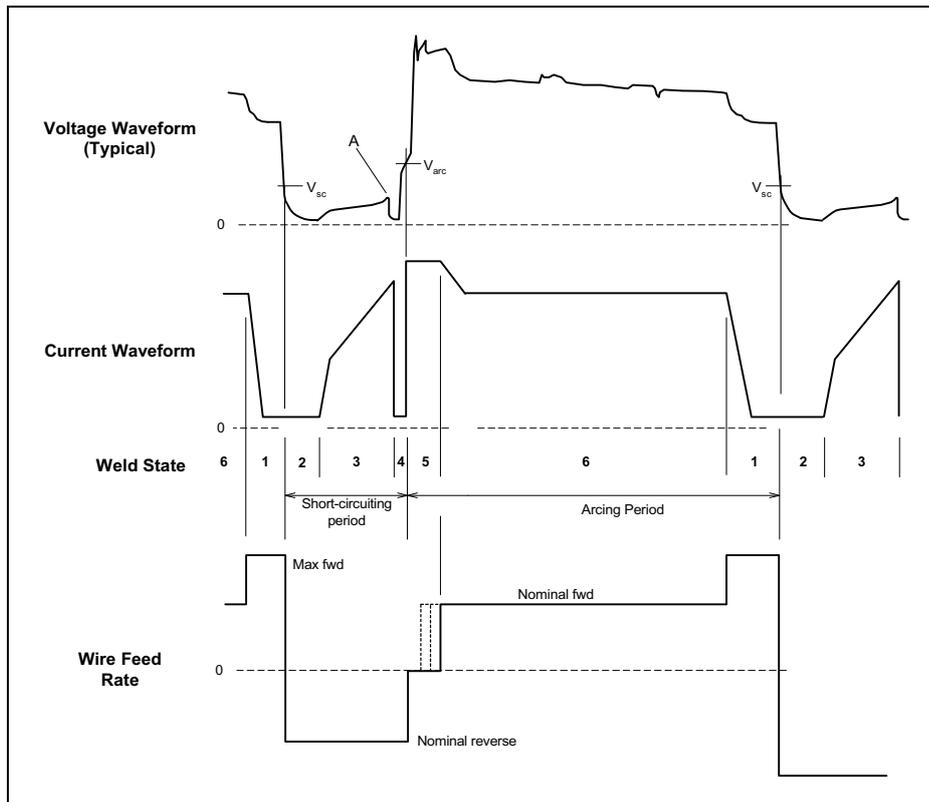
**Figure 10 Typical waveforms for current, wire feed speed, and welding voltage**
