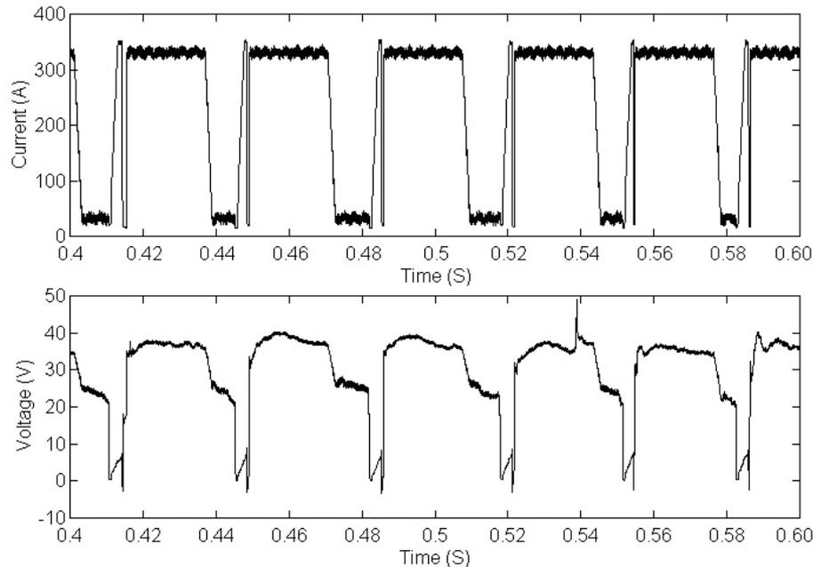
**Figure 11 Voltage and current waveforms for weld at  $I_{\text{mean}}=240\text{A}$**
