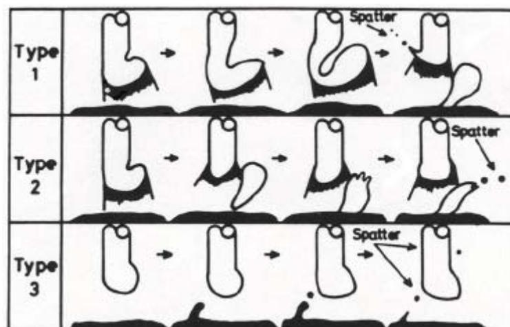
Figure 6 Observed spatter production mechanisms in pulsed CO<sub>2</sub> welding (from [15])
