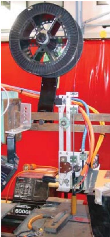
Figure 8 Reversing wire feed unit
