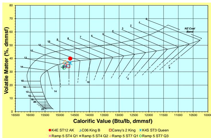
**Figure 3: Suggate rank plot of coal samples from Meandu Min**
