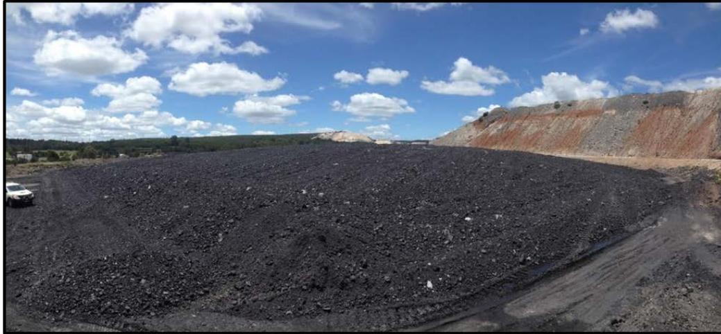
**Figure 6: Carey’s low ash “Enviro” coal stockpile, track rolled in several lifts and batters reduced to limit ingress of air in line with SOP 4868-SE-SOP1027 (“Spon Com”) guidelines**
