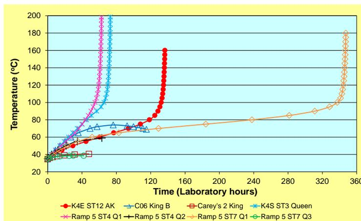
Figure 5: Adiabatic incubation test results for coal samples from Meandu Mine
