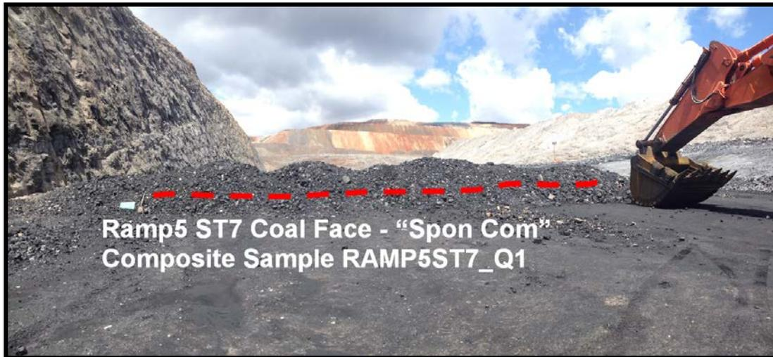
**Figure 2: Sampled coal material from Ramp 5 ST7 for spontaneous combustion testing**
