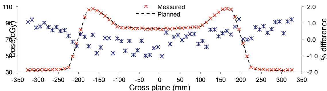
**Figure1:** Planned and measured dose profiles along the X direction for the simple plan delivered without error
