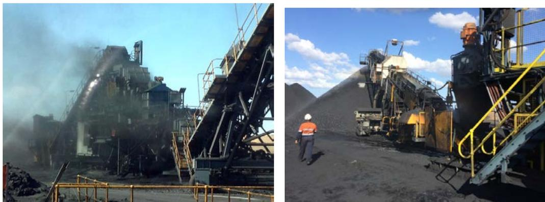
**Figure 9: Mobile crushing station (before and after dust suppression)**
