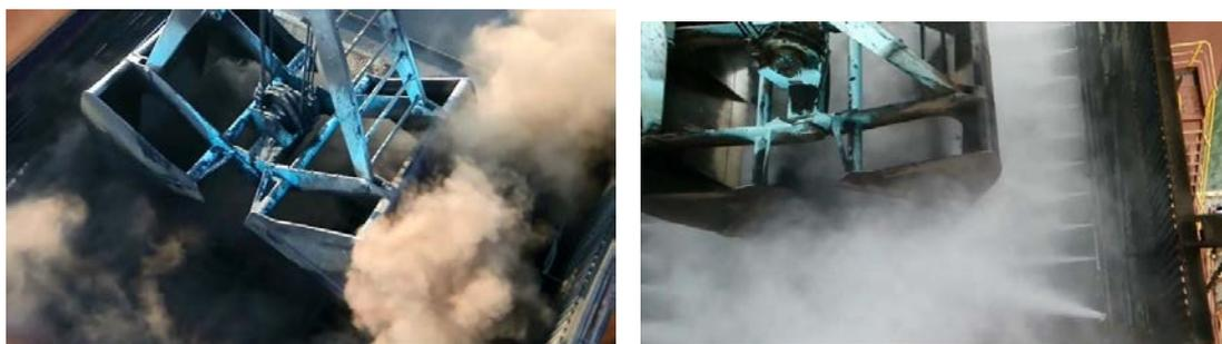
Figure 12: Grab bucket ship unloading (before and after dust suppression)
