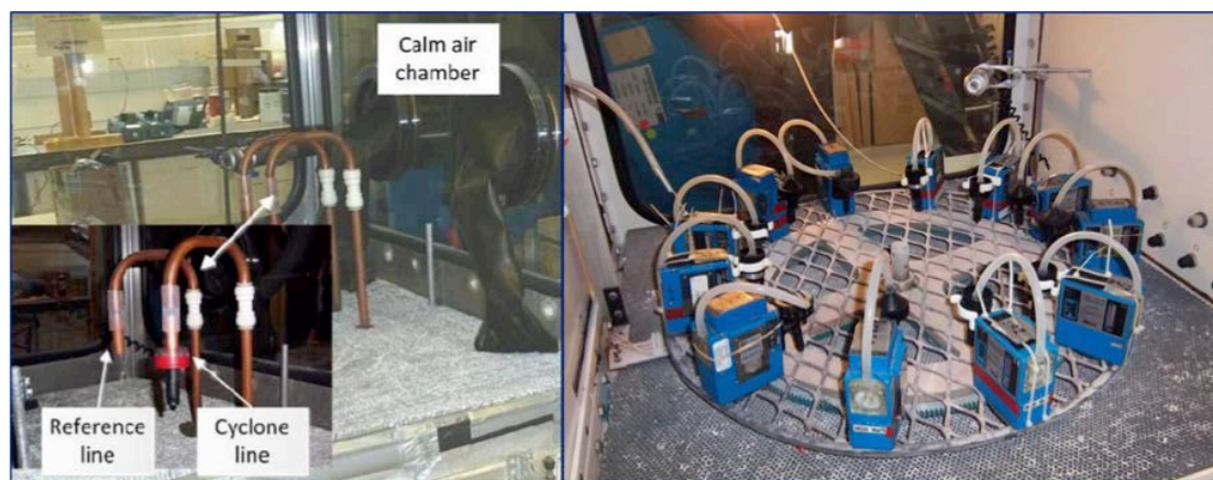
Figure 4: Cyclone sampler testing (left) and dust concentration experimental test set up (Source, HSE, 2016).
