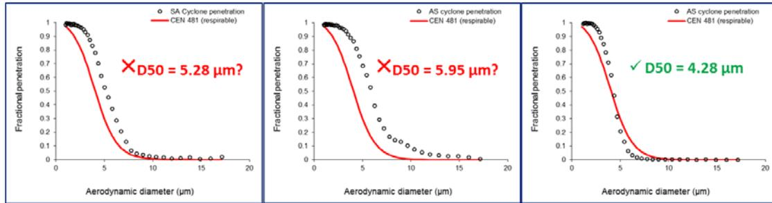
**Figure 5: Fractional penetration average of particles through South African (left), Australian (middle) and UK SIMPEDS cyclone (Right) gravimetric samplers as a function of aerodynamic particle diameter (HSE, 2016).**
