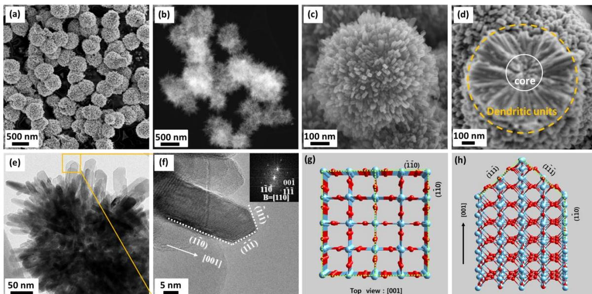
**Figure 1.** (a) Low magnification SEM image and (b) DF STEM image of 3D hierarchical rutile  $\text{TiO}_2$  architecture (HRTA). (c) SEM image of an individual HRTA microsphere. (d) SEM image of a fractured microsphere. (e) TEM image of a quarter microsphere. (f) TEM image of individual nanorod; inset: corresponding SAED pattern. (g, h) atomic structure of a rutile nanorod.
